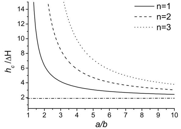
Fig. 2. Normalized microwave threshold field as a function of the elliptic cylinder aspect ratio
