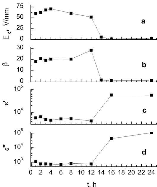
**Fig. 5.** Dependences of the electric field at the classification voltage across a specimen (a), the CVC nonlinearity coefficient (b), and the real (c) and imaginary (d) parts of the complex dielectric permittivity (at  $f = 10^5$  Hz) on the sintering time
