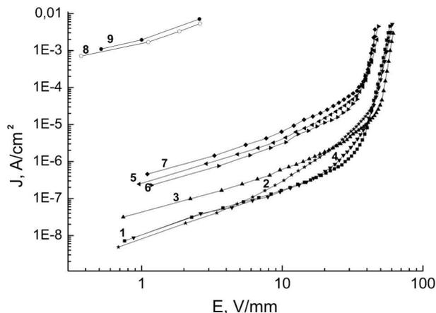
**Fig. 4.** Current-voltage characteristics for a specimen of the varistor ceramics sintered for various times: 1 (1), 2 (2), 3 (3), 4 (4), 6 (5), 8 (6), 12 (7), 16 (8), and 24 h (9)
