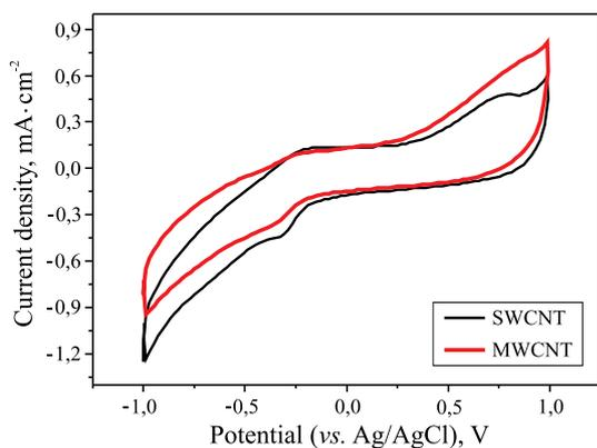
**Fig. 3.** CVs recorded for aqueous SWCNT and MWCNT suspensions (1.0 KCl) on a GC electrode (0.24 cm<sup>2</sup>) at  $v = 0.10 \text{ V} \cdot \text{s}^{-1}$
