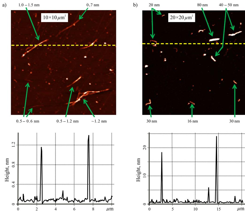
**Fig. 2.** AFM images of SWCNTs (a) and MWCNTs (b) deposited from an aqueous suspension (concentration: 5 μg/ml) on the mica substrate (tapping mode). Topographic images for a given profile (dashed line) are shown on the top. The diameters of some CNTs are indicated by arrows
