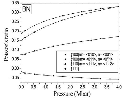
Fig. 8. Poisson's ratio versus the hydrostatic pressure
