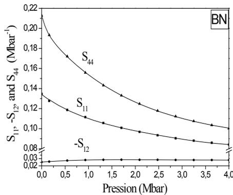
Fig. 6. Compliance constants  $S_{ij}$  versus the hydrostatic pressure
