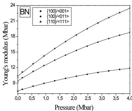
Fig. 7. Young modulus versus the hydrostatic pressure
