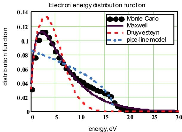
**Fig. 2.** Distribution function of the electron energy at the drift in a uniform electric field ( $E/N = 13.5$  Td, neon). Bullets – the results of Monte Carlo calculations. For comparison, the Maxwell EEDF (solid curve), Druyvesteyn EEDF (dashed curve), and pipe-line distribution (dot-dashed curve) are also given
