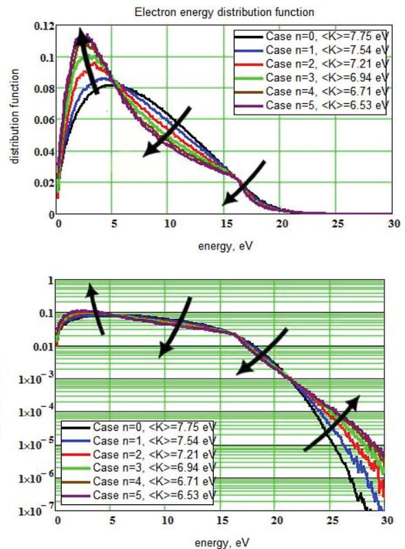
**Fig. 3.** Electron energy distribution in the drift in the periodic electric field ( $E/N = 10$  Td, neon, the field period is equal to 4 cm, field intensity – 4 V/cm). Different curves correspond to different values of the exponent field inhomogeneity. The arrows indicate the direction of changes with the increase of fluctuations of the field
