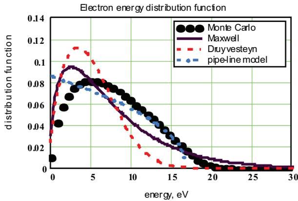
**Fig. 1.** Electron energy distribution function (EEDF) at the drift in a uniform electric field ( $E/N = 13.5$  Td, neon). Bullets – the results of Monte Carlo calculations. For comparison, the Maxwell EEDF (solid curve), Druyvesteyn EEDF (dashed curve), and pipe-line distribution (dot-dashed curve) are also given
