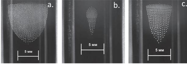
**Fig. 5.** *a* – Ne  $P = 80$  Pa, air  $P = 10$  Pa, particles are 4.83 micrometers in size. *b* – Ne  $P = 80$  Pa, particles are 3.38 micrometers in size. *c* – Ne  $P = 80$  Pa, air  $P = 10$  Pa, particles are 3.38 and 4.83 microns in size
