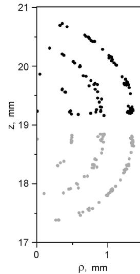
Fig. 4. Special distribution of particles in Coulomb balls. Projection of the spherical coordinates on the plane. Radius of black particles is 2.4 microns. Radius of grey particles is 2.41 microns
