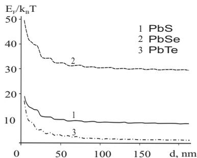
Fig. 2. Calculated values of the Fermi energy  $E_F$  in units of  $k_B T$  versus the QW width for PbS, PbSe, and PbTe at  $T = 300$  K
