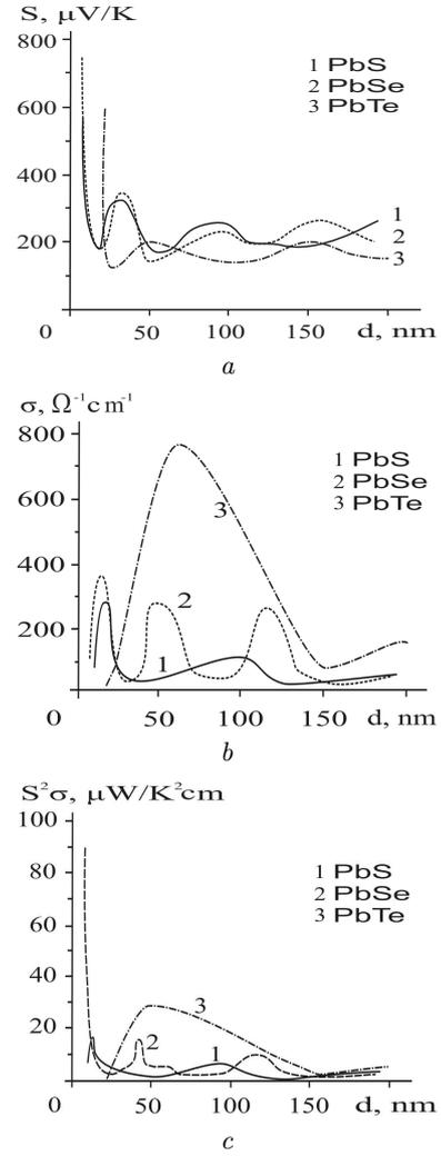
**Fig. 1.** Experimental dependences of the Seebeck coefficient  $S$  (a), electric conductivity  $\sigma$  (b), and TE power factor  $S^2\sigma$  (c) on the thickness of the nanofilms of PbS, PbSe, and PbTe on the substrate of KCl covered with a layer of EuS, at  $T = 300$  K [3–5]
