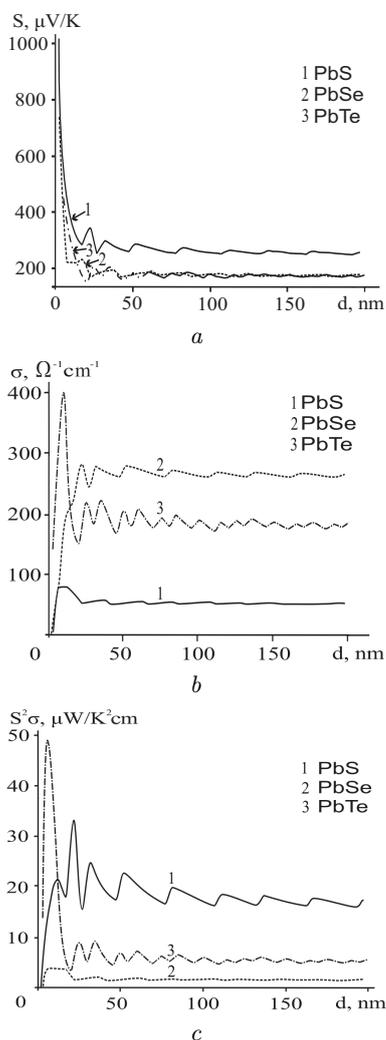
Fig. 3. Theoretical dependences of the Seebeck coefficient  $S$  (a), electric conductivity  $\sigma$  (b), and TE power factor  $S^2\sigma$  (c) on the QW width for films of PbS (1), PbSe (2), PbTe (3) in the model of infinitely deep potential well at  $T = 300$  K
