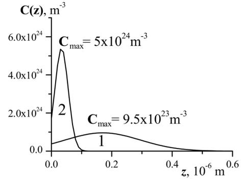
Fig. 5. Profiles of implant distribution in typical Cd<sub>x</sub>Hg<sub>1-x</sub>Te/CdZnTe ( $x \approx 0.223$ ) structures implanted with (1) boron and (2) silver ions
