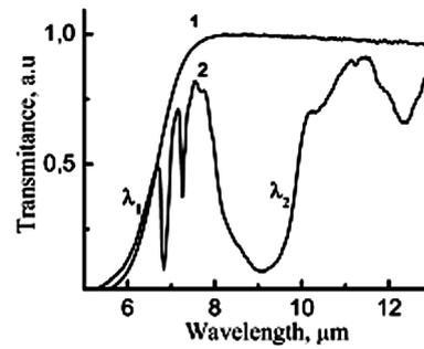
**Fig. 3.** Transmission spectra of a typical Cd<sub>0.223</sub>Hg<sub>0.777</sub>Te/CdZnTe specimen (a) in the initial state and (b) after implantation with boron and annealing
