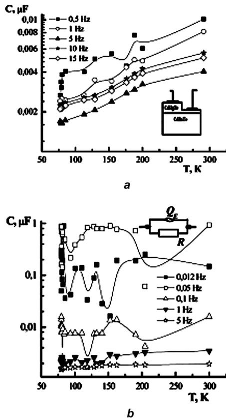
**Fig. 4.** Temperature dependences of the capacitance of typical  $\text{Cd}_{0.223}\text{Hg}_{0.777}\text{Te}/\text{CdZnTe}$  structures implanted with (a)  $\text{B}^+$  and (b)  $\text{Ag}^+$  and measured at various frequencies of the excitation signal. The inset in panel (a) demonstrates the scheme of the examined mesostructure fabricated with the use of the method of chemical etching, and the inset in panel (b) shows the corresponding equivalent circuit
