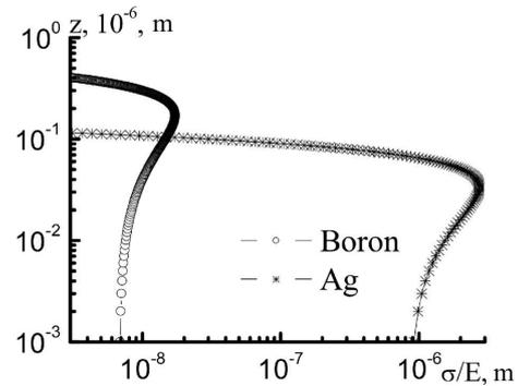
Fig. 6. Profiles of deformations in the Cd<sub>0.223</sub>Hg<sub>0.777</sub>Te film on the CdZnTe substrate induced by introducing the B<sup>+</sup> and Ag<sup>+</sup> impurities
