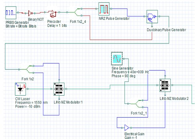
Fig. 4. Transmitter design for the duobinary modulation format
