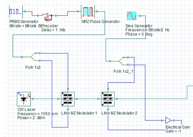
Fig. 3. Transmitter design for DPSK
