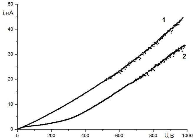
Fig. 3. Current-voltage dependences of the dark (1) and X-ray conductivities (2) of a single-crystal ZnSe specimen at room temperature
