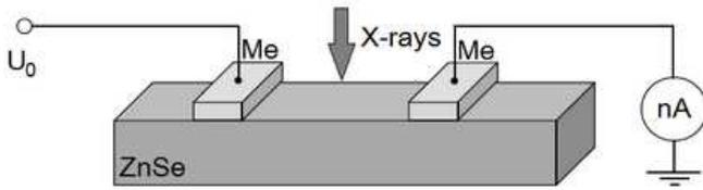
Fig. 1. Scheme of measurements of the X-ray conductivity
