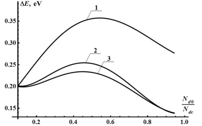
Fig. 2. Dependences of the electron energy difference  $\Delta E$  between the first excited and ground states in a GaAs/InAs/GaAs heterostructure with a defect nanocluster in the InAs quantum well on the average defect concentration at  $m_3/m_0 = 0.03$  (1), 0.07 (2), and 0.09 (3)
