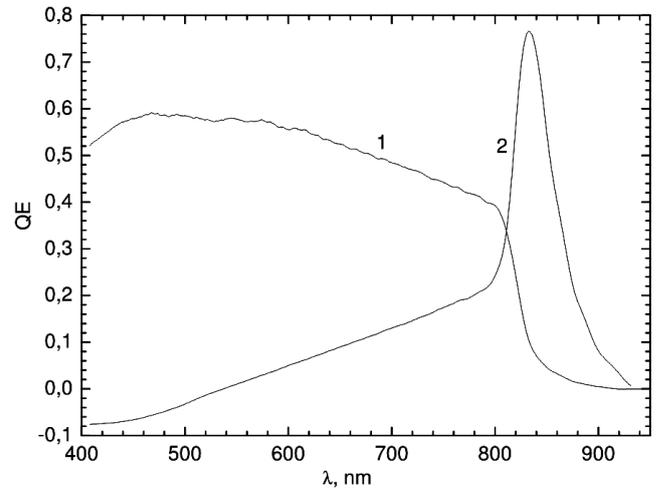
Fig. 4. Spectral dependences of a condenser photo-emf signal normalized to a constant number of light-flux quanta obtained for the ITO/CdTe structure preliminarily annealed in air at  $T = 430$  °C: (1) the initial spectral dependence, (2) after the hydrogen treatment and the DLCF deposition
