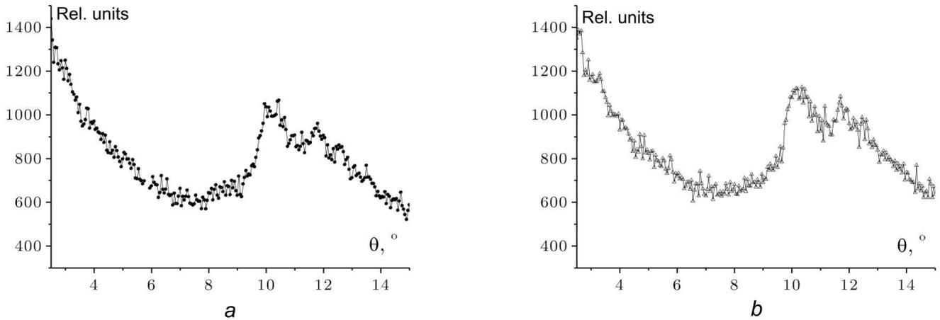
Fig. 3. Angular dependences of the intensity of X-ray radiation diffracted at untreated (a) and treated (b) specimens. The specimen axes are oriented along the meridian
