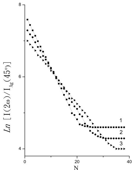
Fig. 2. Kinetics of molecular desorption from the Cu surface for different values of energy density of the incident radiation: 1 – 350, 2 – 300, 3 – 260 J/m<sup>2</sup>
