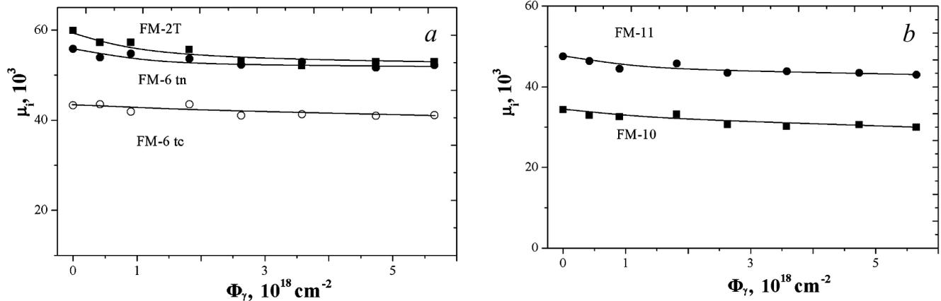
Fig. 2. Dose dependences of the initial magnetic permeability ( $f = 10$  kHz) of magnetic circuits fabricated from FM-alloys
