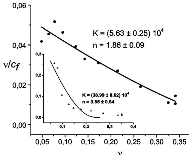
Fig. 9. Approximation for the non-cooperative binding by the McGhee–von Hippel equation and in the Scatchard coordinates. The same, but in the case where  $A_b$  was determined without the approximation of initial data, is depicted in the inset
