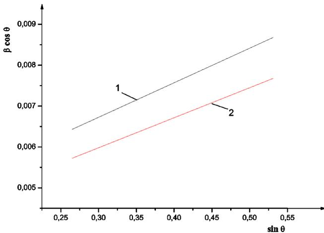
Fig. 4. Williamson-Hall plots at the approximation by the Cauchy function for specimens with a deposition time of 45 (1) and 60 min (2)
