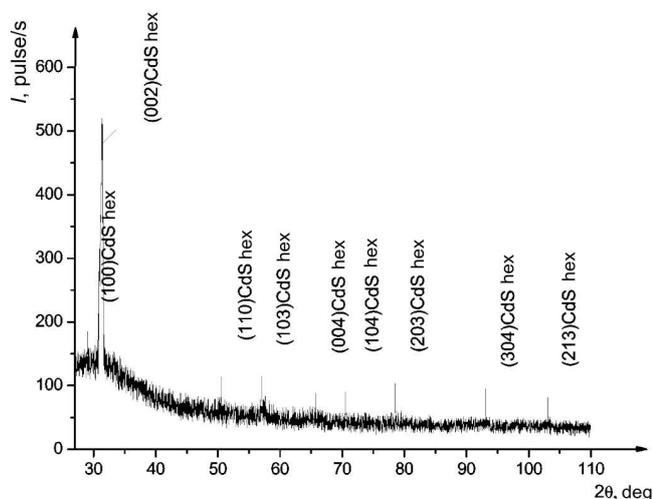
Fig. 1. X-ray diffraction pattern of a CdS film fabricated by the hot-wall technique with a deposition time of 35 min
