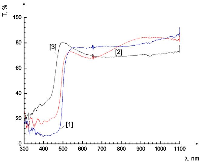
Fig. 6. Dependences of the transmittance coefficient on the wavelength for glass/CdS specimens fabricated by the hot-wall technique with various deposition times of 35 (1), 45 (2), and 60 min (3)
