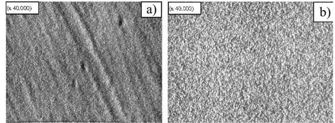
Fig. 5. Micrographs of the surfaces of cadmium sulfide films 0.14 (a) and 0.21 μm (b) in thickness
