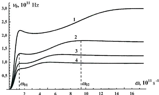
Fig. 3. Dependences of the modulation amplitude for the recombination radiation frequency which corresponds to the transition between the ground states of an electron and a hole in the InAs/GaAs heterostructure with InAs quantum dots on the acoustic wave frequency for various quantum dot dimensions  $R_0 = 3$  (1), 5 (2), 7 (3), and 9 nm (4)
