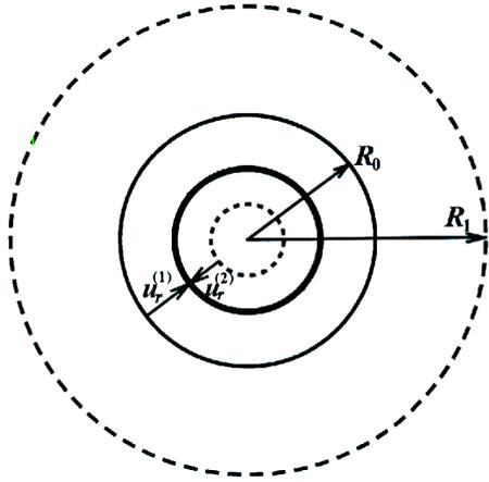
Fig. 1. Model of a strained spherical quantum dot.  $u_r^{(i)}$  are the radial components of shift vectors in the quantum dot ( $i = 1$ ) and matrix ( $i = 2$ ) materials
