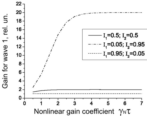
Fig. 4. Gain coefficient for wave 1,  $I_1^{out}/I_1$ , at various ratios  $I_1/I_2$  between input-wave intensities
