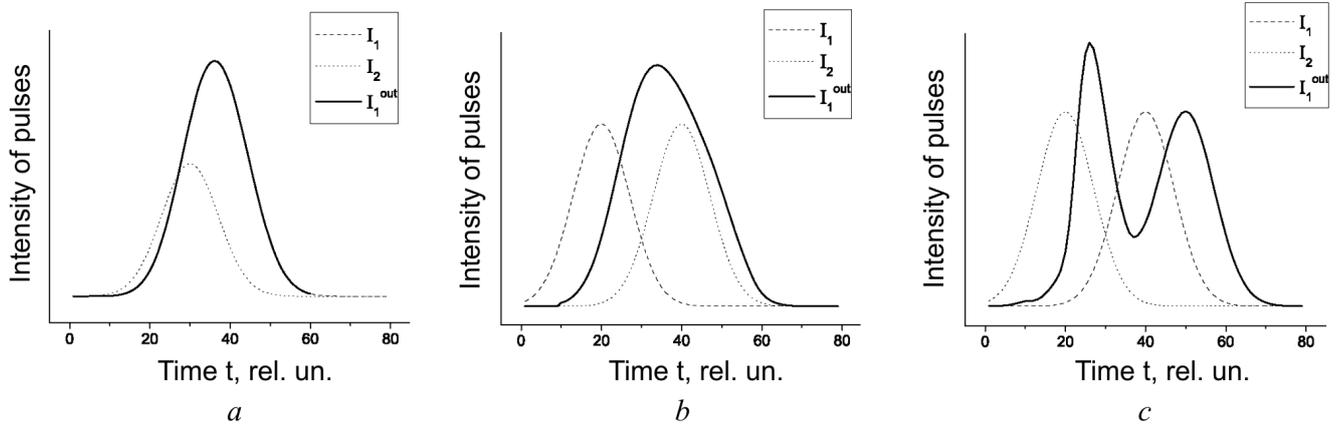
Fig. 6. Transformation of the pulse shape at the medium output,  $I_1^{\text{out}}$ , induced by the interaction between two Gaussian input beams ( $I_1, I_2$ ) in a nonlinear medium with a nonlocal response in the reflection geometry. The time delays between the input pulses: (a) input beams are synchronized ( $\Delta_1 = \Delta_2$ ), (b)  $\Delta_1 < \Delta_2$ , and (c)  $\Delta_1 > \Delta_2$
