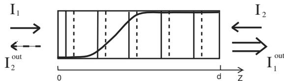
Fig. 1. Diagram of the two-beam interaction in a medium with a nonlocal nonlinear response in the reflection geometry of the problem. Straight lines mark the interference pattern maxima, and dashed ones the maxima of the dynamical refractive-index grating. The curve illustrates the grating amplitude distribution
