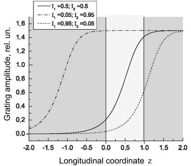
Fig. 5. Stationary distribution of the grating amplitude for input wave intensities presented in Fig. 4. The nonlinear gain coefficient of the medium  $\gamma_N\tau = 3$ . The nonfilled interval  $z = [0,1]$  corresponds to the nonlinear medium bulk ( $d = 1$ )
