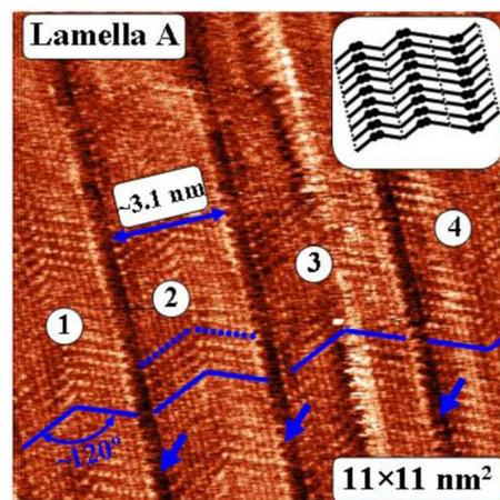
Fig. 4. Intramolecular separation of a monolayer of hexadecyl boron acid on graphite. Lamellae are formed by dimers of molecules of the acid. Polar groups  $-\text{B}(\text{OH})_2$  are located in the middle of each lamella. Spots denote the positions of  $-\text{CH}_2$ -groups of an alkyl chain. Scanning area:  $10 \times 10 \text{ nm}^2$ , tunneling current:  $I_t = 50 \text{ pA}$ , voltage on the gap:  $U_t = 350 \text{ mV}$ . In insert: schematic model of packing
