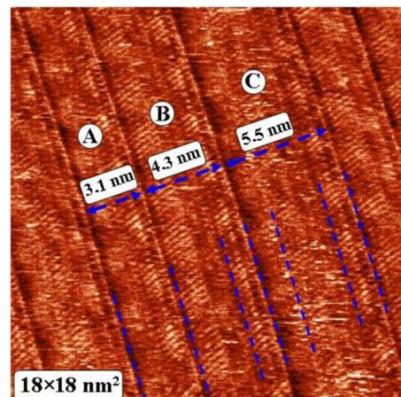
Fig. 3. Lamella-like structure of a monolayer of hexadecyl boron acid on graphite. Three types of lamellae with different widths. Scanning area:  $18 \times 18 \text{ nm}^2$ . Tunneling current:  $I_t = 60 \text{ pA}$ , voltage on the gap:  $U_t = 300 \text{ mV}$
