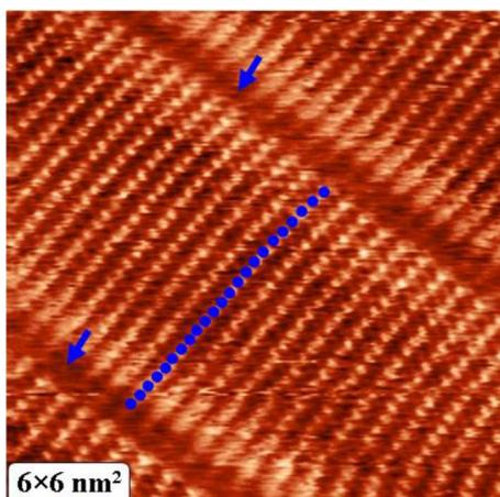
Fig. 5. Intramolecular separation of a monolayer of alkane  $n\text{-C}_{46}\text{H}_{94}$  on graphite. The number of  $\text{-CH}_2\text{-}$  groups visible on the STM-image is equal to 23 (marked by spots), which is twice less than that in a molecule of  $\text{C}_{46}\text{H}_{94}$ . Scanning area:  $6 \times 6 \text{ nm}^2$ , tunneling current:  $I_t = 50 \text{ pA}$ , voltage on the gap:  $U_t = 350 \text{ mV}$
