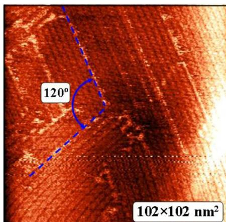
Fig. 2. (a) STM-image of a monolayer of hexadecyl boron acid on the *n*-tetradecane/graphite interface. Scanning area:  $102 \times 102 \text{ nm}^2$ . Tunneling current:  $I_t = 60 \text{ pA}$ , voltage on the gap:  $U_t = 350 \text{ mV}$
