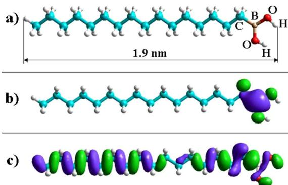
Fig. 1. (a) – Structure of a free neutral molecule of hexadecyl boron acid optimized by the density functional method. (b) and (c) – profiles of the first empty (LUMO+1) and filled (HOMO-1) molecular orbitals close to the Fermi level for a free neutral molecule of hexadecyl boron acid, which are calculated within the method DFT/B3LYP/6-31G\*. The energies  $E = 1.79$  eV (b) and  $E = -8.01$  eV (c)
