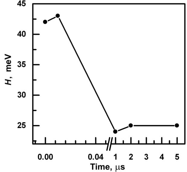
Fig. 6. Time dependences of the half-width  $H$  of the PL zero-phonon line of a 5/5 SL at high levels of excitation.  $T = 5$  K
