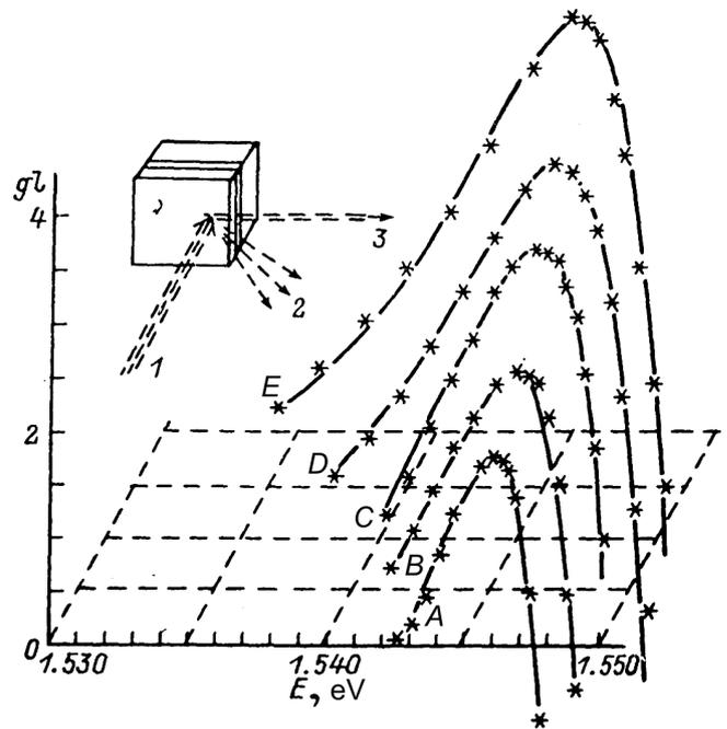
Fig. 8. Optical gain spectra of the GaAs/Al<sub>0.35</sub>Ga<sub>0.65</sub>As SL at various exciting emission densities  $L$ . Points – experiment ( $T = 4.2 \text{ K}$ ,  $l = 100 \mu\text{m}$ ), continuous curves – calculations.  $L$  (MW/cm<sup>2</sup>): *a* - 0.2, *b* - 0.44, *c* - 0.76, *d* - 1.68, *e* - 4. The insert shows the geometry of the experiment. 1 - laser beam, 2 - spontaneous emission, 3 - stimulated emission
