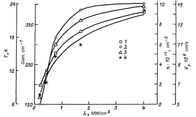
Fig. 9. Dependence of the fitting parameters on the excitation power density  $L$ : the density of electron-hole pairs  $n$  (1), temperature  $T$  (2), drift velocity  $V_D$  (3), and the coefficient of optical gain  $g$  (4), which are used at the fitting of experimental and theoretical curves  $g(E)$  (Fig. 8)
