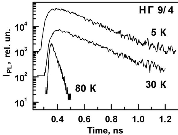
Fig. 3. Time variations of the PL maximum intensity of a 9/4 SL at  $T = 5, 30,$  and  $80$  K
