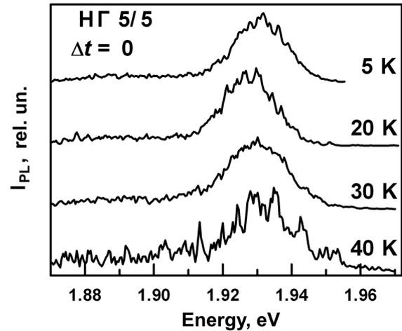
Fig. 4. TRPL spectra of a 5/5 SL at the zero delay after the exciting pulse ( $\Delta t = 0$ ) at various temperatures
