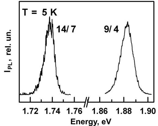
Fig. 2. PL spectra of 14/7 and 9/4 SLs at  $T = 5$  K. Spectra are normed to their maxima
