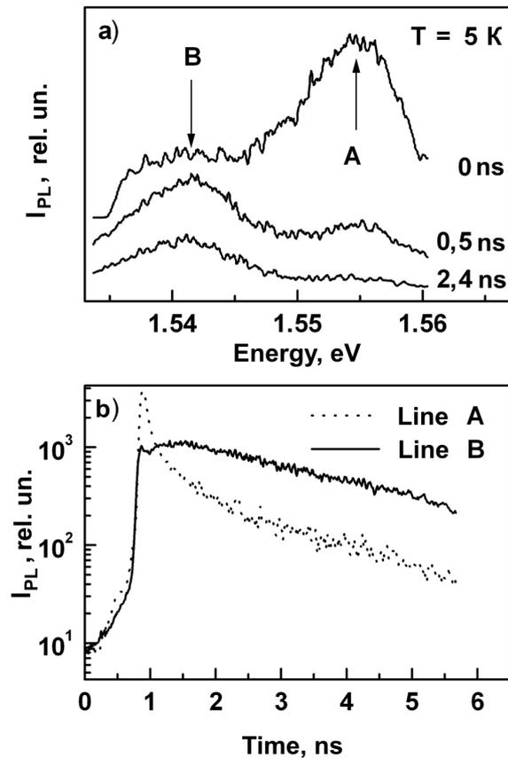
Fig. 1. (a) PL spectra of a 36/36 SL at  $T = 5$  K obtained at various time delays after the exciting pulse; (b) the time behavior of the PL intensities of lines A and B
