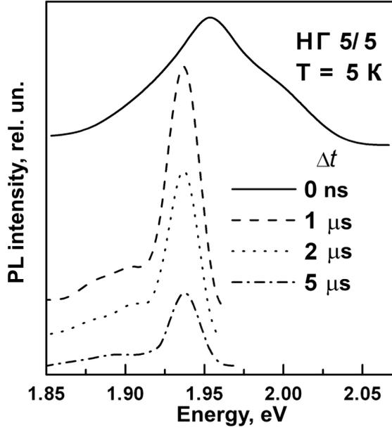
Fig. 5. PL spectra of a 5/5 SL obtained at various time delays for high levels of excitation
