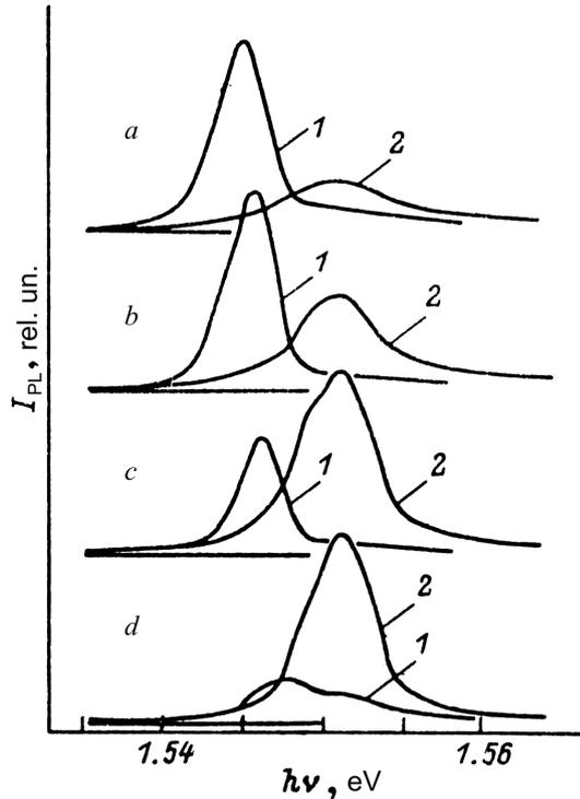
Fig. 7. Spectra of stimulated (1) and spontaneous (2) emissions of the GaAs/Al<sub>0.35</sub>Ga<sub>0.65</sub>As SL at various excitation power densities ( $L_0 = 4 \text{ MW/cm}^2$ ). *a* -  $L_0$ , *b* -  $0.2L_0$ , *c* -  $0.05L_0$ , *d* -  $0.02L_0$
