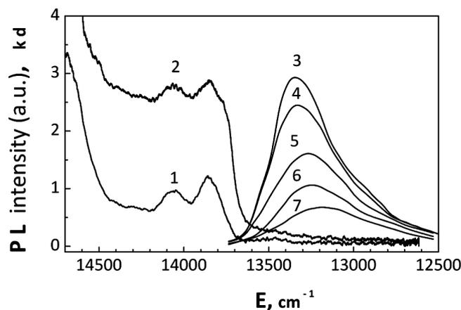
Fig. 1. Absorption, for *B*- (2) and *A*- (1) polarizations, and photoluminescence, at temperatures  $T = 4.2$  (1–3), 14 (4), 20 (5), 25 (6), and 30 K (7), spectra for a pentacene single crystal with the thickness  $d = 20$   $\mu\text{m}$ . The PL spectra were measured from the smooth surface,  $\lambda_e = 441.6$  nm
