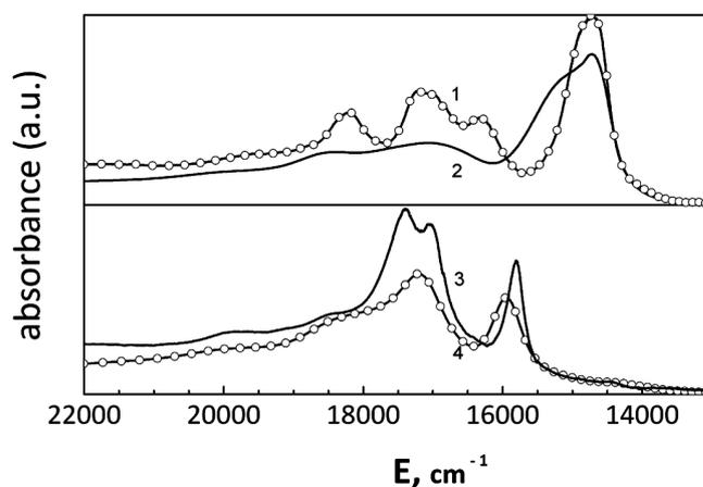
Fig. 3. Absorption spectra for a single-crystalline pentacene film of the thickness  $d = 100 \text{ nm}$ , which is in the optical contact with a quartz substrate, for the  $B$ - (1 and 2) and  $A$ - (3 and 4) polarizations at  $T = 42$  (1 and 3) and 296 K (2 and 4)
