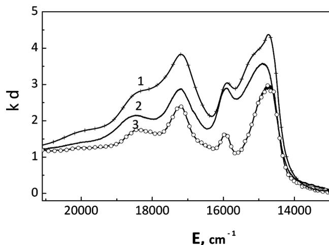
Fig. 4. Absorption spectra for a single-crystalline pentacene film (1) and a pentacene film obtained by thermal sputtering in vacuum (2 and 3). The film thickness  $d = 100$  nm. Measurements were carried out in natural light at  $T = 296$  (1 and 2) and 4.2 K (2)
