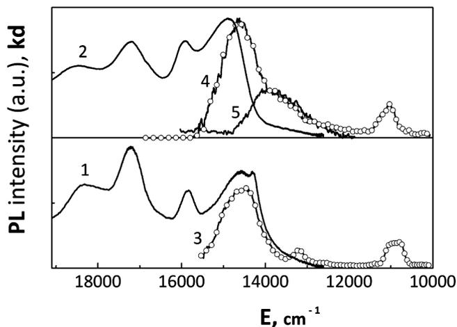
Fig. 5. Absorption (1 and 2) and photoluminescence (3–5) spectra of a thermally sputtered pentacene film with the thickness  $d = 100$  nm at temperatures  $T = 4.2$  (1 and 3) and 296 K (2, 4, and 5).  $\lambda_e = 532$  (3 and 4) and 337.1 nm (5)
