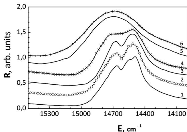
Fig. 2. Reflection spectra for the  $B$ -polarization of a freely fixed pentacene single crystal at various temperatures  $T = 1.85$  (1), 4.2 (2), 10 (3), 43 (4), 200 (5), and 250 K (6).  $d = 20 \mu\text{m}$
