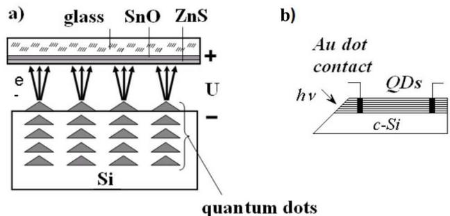
Fig. 2. (a) Diode cell for measuring the field emission and the field-enhanced photoemission of electrons. (b) Specimen for photoconductivity measurements
