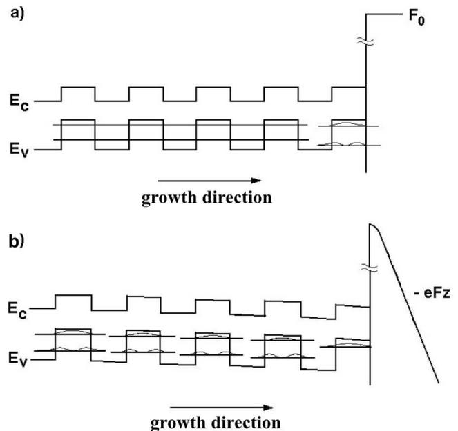
Fig. 4. Energy band structure of a Si/SiGe heterojunction (a) without and (b) with the applied electric field  $F = 10^6$  V/cm
