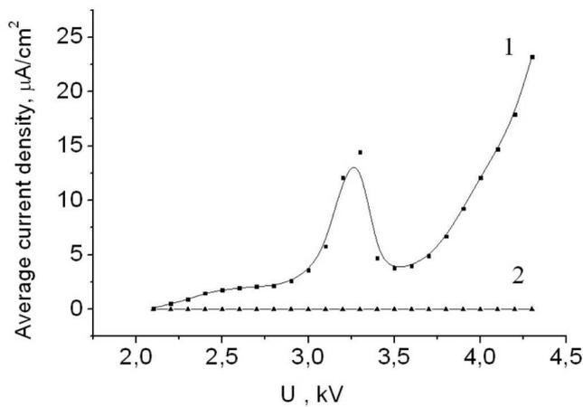
Fig. 3. (1) Current-voltage characteristic of the field-enhanced photoemission from a Si/Ge heterostructure with 5 layers of QDs about 2 nm in height. (2) Current-voltage characteristic of the dark field emission for the same heterostructure
