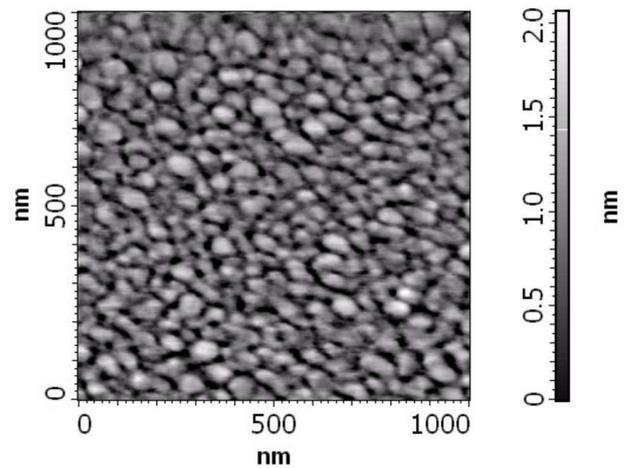
Fig. 1.  $1 \times 1\text{-}\mu\text{m}^2$  AFM image of a structure with QDs at  $500 \text{ }^\circ\text{C}$ . The average height and lateral size of QDs are about 2 and 30 nm, respectively
