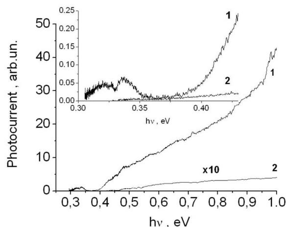
Fig. 5. Spectral dependences of the lateral photoconductivity of a Ge/Si heterostructure with Ge quantum dots measured at the lateral excitation (1) and the normal incidence of light (2) at a temperature of 77 K. The inset details the low-energy section of the spectra
