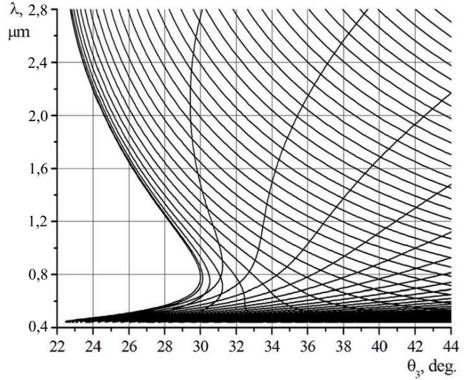
Fig. 7. Family of tuning curves for the OPG process in a BBO crystal
