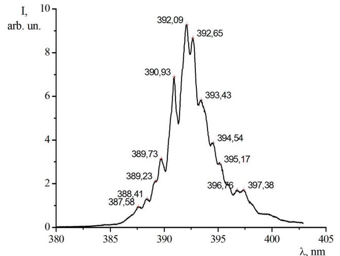
Fig. 4. Spectrum of the central zone of radiation at the output of a BBO-2 crystal sample pumped with the second harmonic of a Ti:Sa femtosecond laser
