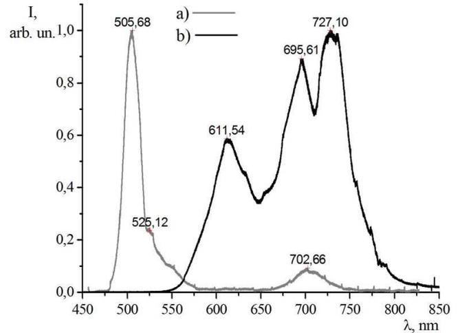
Fig. 5. Spectrum of the ring zone of radiation. a – for BBO-3 crystal sample; b – for BBO-2 crystal sample
