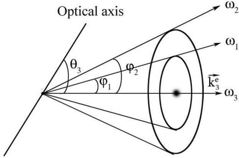
Fig. 6. Scheme of propagation of the pumping  $\omega_3$ , signal  $\omega_1$ , and idler  $\omega_2$  waves under conditions of the non-collinear synchronism
