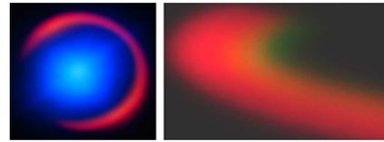
Fig. 3. Radiation at the output of a BBO-2 sample, pumped with the second harmonic of a Ti:Sa laser: a – general view of the output radiation; b – detailed view of the ring zone of the output radiation obtained using a prism
