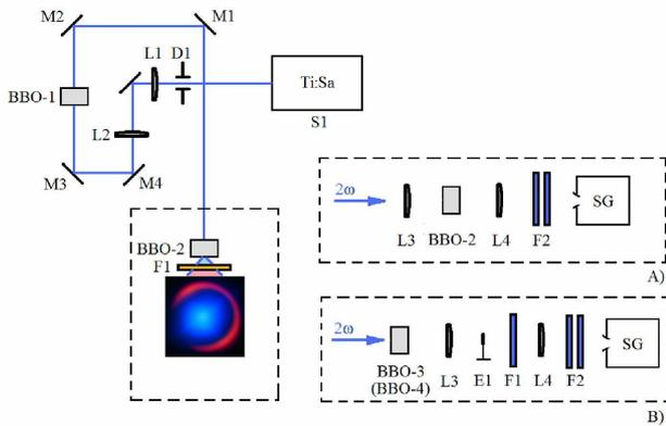
Fig. 1. Experimental setup used in the present work. S1 – source of femtosecond laser pulses; BBO-1 – BBO crystal sample for the second harmonic generation; BBO-2, BBO-3, BBO-4 – BBO crystal samples of different orientations utilized for the investigation of laser light scattering; SG – spectrograph SP-2558 (groove density – 1200 g/mm); L1..L4 – lenses; F1, F2 – filters; E1 – shield; D1 – diaphragm
