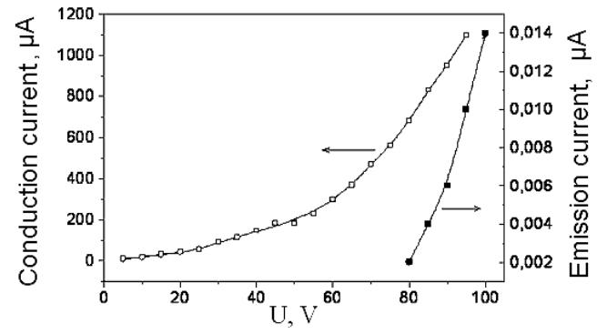
Fig. 4. Current-voltage characteristic of conduction and emission currents from dispersed C-nanotubes
