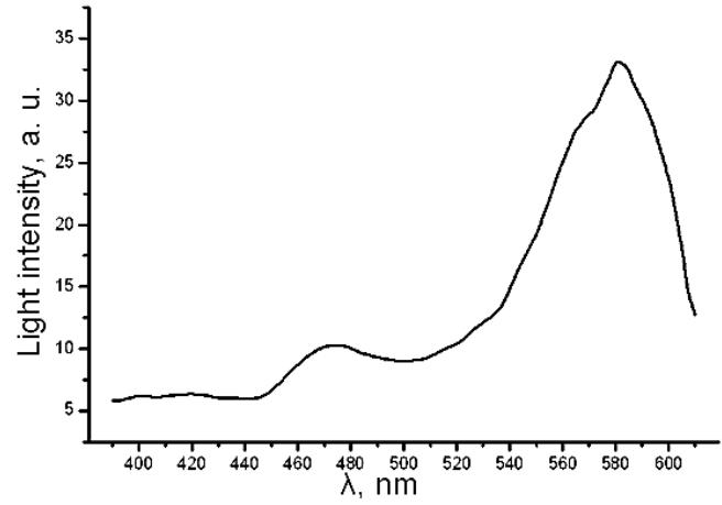
Fig. 5. Spectrum of photon emission from dispersed C-nanotubes
