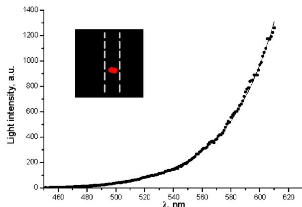
Fig. 2. Photon emission spectrum recorded at the voltage  $U = 3$  V. Inset: the image of the luminescence (hatched area) of a bunch of initial C-nanotubes between metal film contacts shown by a dashed line
