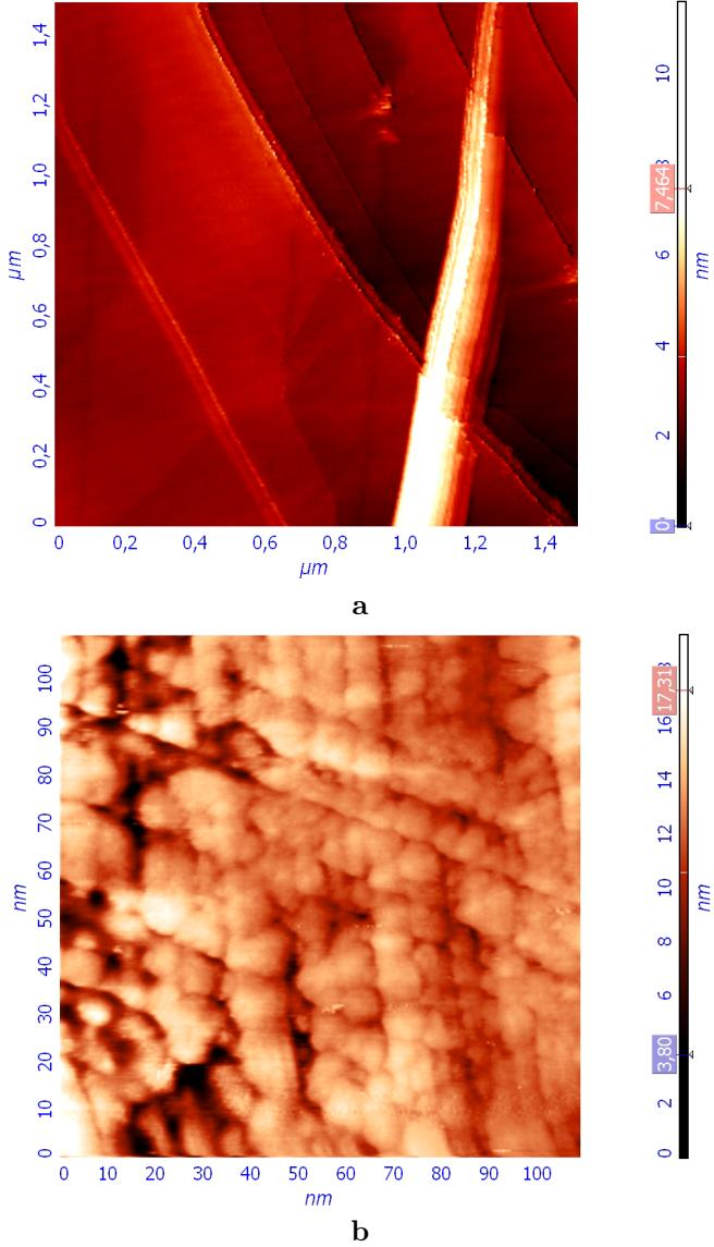
Fig. 3. STM image of C-nanotubes before (a) and after (b) their dispersion
