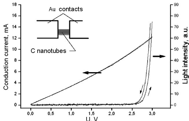
Fig. 1. Conduction current-voltage characteristic of a bunch of initial C-nanotubes and the photon emission intensity as a function of the applied voltage. Inset: the schematic of an experimental sample
