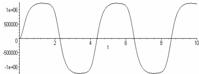
Fig. 4. Dependence  $J(t)$  for a sinusoidal external field corresponding to the hysteresis loop shown in Fig. 3
