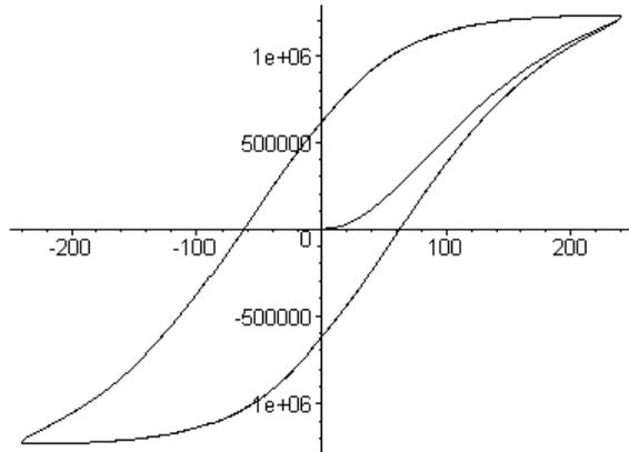
Fig. 3. Dynamical hysteresis loop in a typical ferromagnetic in the coordinates  $J - H$  [A/m]
