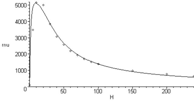
Fig. 1. Experimental points and curve (8) approximating the experimental dependence of the magnetic permeability  $\mu(H)$  ( $\mu_{\max} = 5170$ ,  $H$  [A/m])
