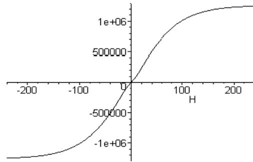
Fig. 2. Basic curve of magnetization  $J_0(H)$  corresponding to the magnetic permeability shown in Fig. 1 ( $J, H$  [A/m])
