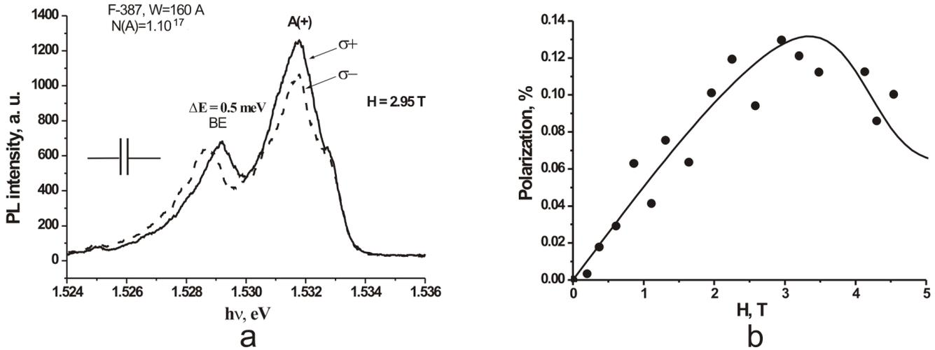
Fig. 2. PL spectrum for two directions of the circular polarization (a), and the dependence of the polarization degree of the right peak on the magnetic field (b). Solid curve – calculation, dots – experiment
