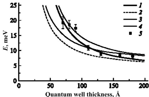
Fig. 1. Dependence of the activation energy of  $A(+)$ -centers on the quantum well thickness. Curves correspond to the energies  $E_1$  and  $E_2$  in the bulk: 1 and 2 –  $E_1=5$  meV,  $E_2=5$  meV, 3 and 4 –  $E_1=7$  meV,  $E_2=7$  meV. Dots – experiment
