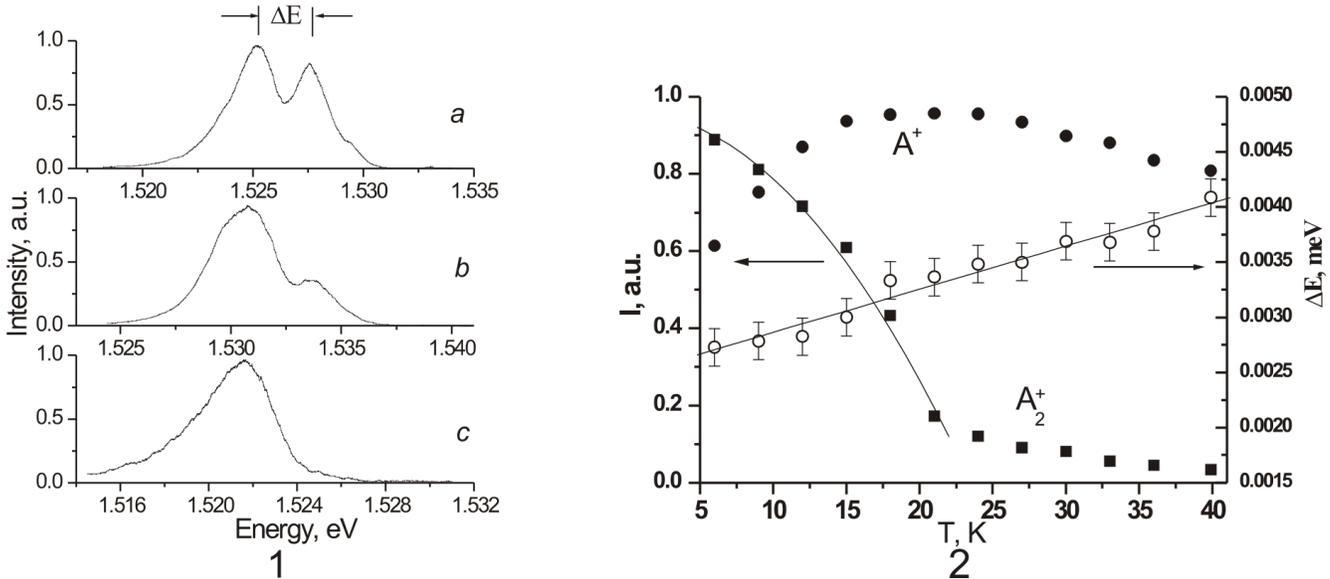
Fig. 3. 1 – Spectra of the samples with various doping levels: a –  $1.5 \times 10^{10}$ , b –  $6 \times 10^{10}$ , and c –  $1.8 \times 10^{11}$   $\text{cm}^{-2}$ . 2 – Temperature dependences of the peak amplitudes of  $A^+$  atomic and  $(A^+)_2$  molecular states
