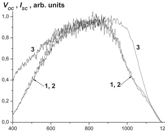
Fig. 3. Spectral dependences of the open-circuit voltage (curve 1) and the short-circuit current (curves 2 and 3), normalized by the corresponding maximal value and the constant flux density of incident quanta, for SC specimens with non-Ohmic (curves 1 and 2) and Ohmic (curve 3) rear contacts and fabricated on the basis of silicon with the  $n$ -type conductivity
