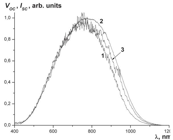
Fig. 4. Spectral dependences of the open-circuit voltage at  $V_{max} \approx 0.3$  mV (curve 1) and  $V_{max} \approx 3.5$  mV (curve 2) and short-circuit current (curve 3), normalized by the corresponding maximal value and the constant flux density of incident quanta, for SCs with non-Ohmic rear contact and fabricated on the basis of silicon with the  $p$ -type conductivity
