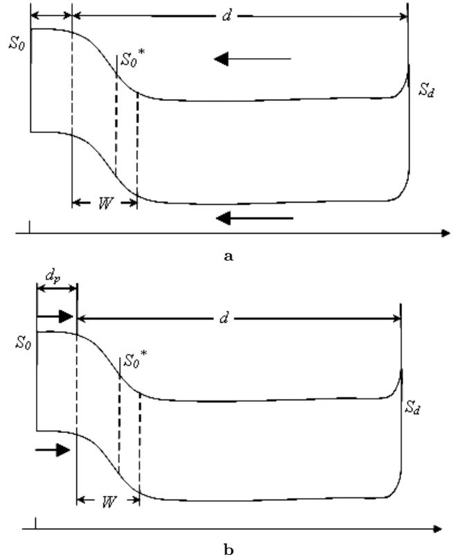
Fig. 5. Schematic energy diagrams for a photosensitive structure with  $n$ -base and planes, in which the surface recombination and recombination in the SCR occur, in the cases where the bulk (a) ( $\alpha(d_p + w) \ll 1$ ) or surface (b) ( $\alpha d_p \gg 1$ ) optic generation dominates
