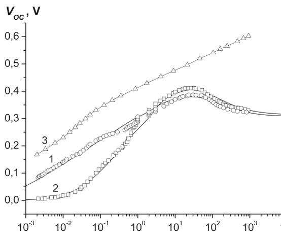
Fig. 2. Dependences of the open-circuit voltage on the specimen irradiance for silicon photosensitive structures fabricated on the basis of a substance with the *n*-type conductivity, and with non-Ohmic (curves 1 and 2) and Ohmic (curve 3) rear contacts. Points denote experimental data, curves 1 and 2 are the results of theoretical simulations
