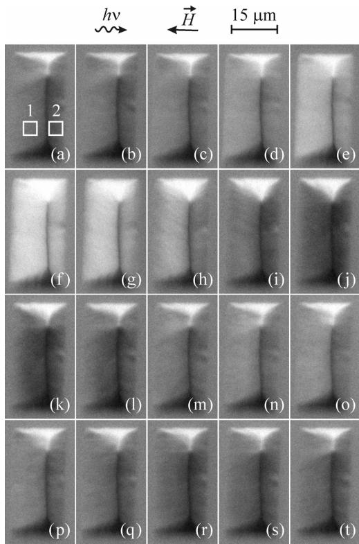
Fig. 3. XMCD-PEEM images of the particle being studied under the action of external magnetic field I at time  $t = 0$  (a), 100 (b), 200 (c), 300 (d), 400 (e), 500 (f), 600 (g), 700 (h), 800 (i), 900 (j), 1000 (k), 1100 (l), 1200 (m), 1300 (n), 1400 (o), 1500 (p), 1600 (q), 1700 (r), 1800 (s), and 1900 ps (t). Designations used here are identical to those in Fig. 1,a
