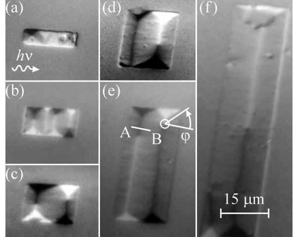
Fig. 2. Static XMCD-PEEM images of the domain structure in the magnetic-field-free state of permalloy rectangular particles 10 nm thick with a lateral size of 16  $\mu\text{m}$  along the horizontal and the aspect ratio of 1:4 (a), 1:2 (b), 3:4 (c), 1:1 (d), 2:1 (e), and 4:1 (f). The magnetic contrast is due to XMCD at the Ni  $L_3$  edge ( $h\nu=853$  eV). Other designations are given in the text
