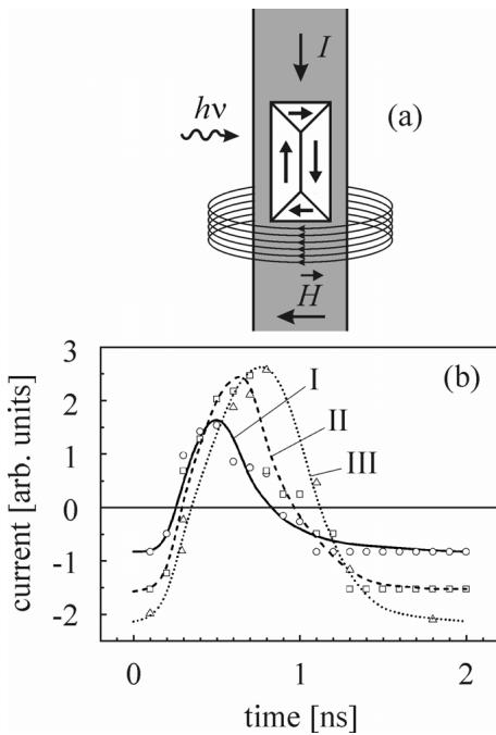
Fig. 1. (a) Scheme of a two-dimensional rectangular permalloy particle on a copper microstrip line. Directions of the projection of synchrotron radiation in the particle plane  $h\nu$ , the current passing through the microstrip line  $I$ , and the magnetic field  $H$  created by it are shown. (b) Current profiles reconstructed from a change of the linear size of PEEM images of the particle being studied under the current passage through the microstrip line. The period of pulses is equal to 2 ns
