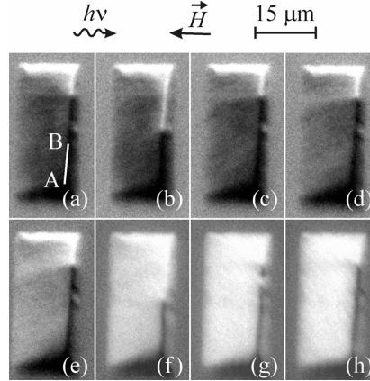
Fig. 4. XMCD-PEEM images of the particle being studied under the action of external magnetic field II at time  $t = 0$  (a), 100 (b), 200 (c), 300 (d), 400 (e), 500 (f), 600 (g), and 700 ps (h). Designations used here are identical to those in Fig. 1,a
