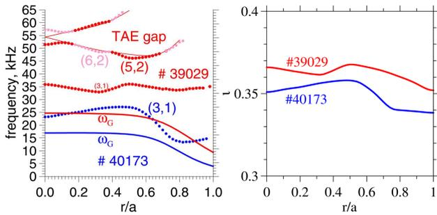
Fig. 3. Continuum branches with given  $(m, n)$  and the geodesic acoustic frequency,  $\omega_G$
