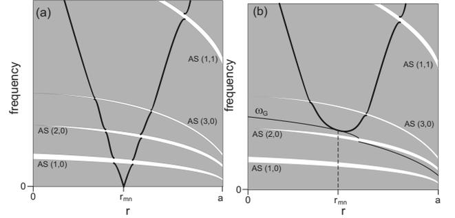
Fig. 1. Alfvén continuum branch: (a)  $\mathfrak{S} \gg 1$  (W7-X case); (b)  $\mathfrak{S} \ll 1$  (W7-AS case). Notations: gray, continuum region, white, Alfvén-sound gaps,  $r_{mn}$  is the  $\iota_{mn}$  radius; AS( $\mu, \nu$ ) denote the Alfvén-sound gaps caused by the Fourier harmonics  $\epsilon_B^{(\mu\nu)}$
