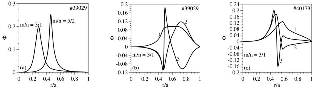
Fig. 2. Calculated AEs in the W7-AS shots #39029 and #40173: (a) GAE in AIs with the lowest frequency (33 kHz) and the highest frequency (46 kHz), respectively, in shot #39029; (b) NGAE in AIs with intermediate frequencies in shot #39029; curve 1, AI with the frequency of 38 kHz; curve 2, 35.3 kHz; curve 3, 35 kHz; (c) NGAEs relevant to AI in shot #40173
