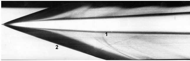
Fig. 2. Temporal photoscan of the channel radius (1) and the radius of shock-wave front (2). Illumination with a parallel light beam from a standard EV-45 source; W = 20 \mu\text{m} , U = 37 \text{ kV} , l = 40 \text{ mm} , and \Delta t = 48 \mu\text{s}
