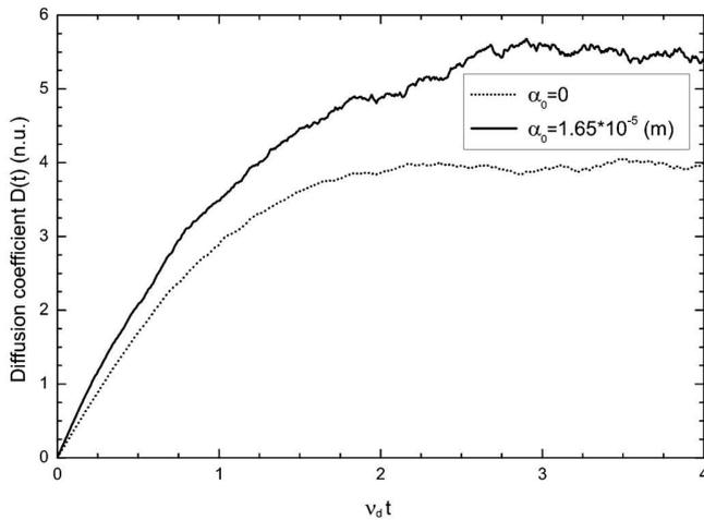
Fig. 5. The time dependence of  $D(t)$  for the standard configuration with magnetic islands (solid line) and without them (dotted line)
