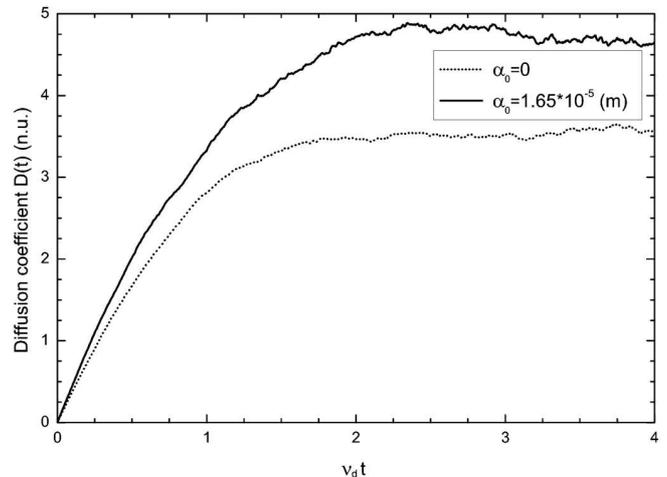
Fig. 6. The time dependence of  $D(t)$  for the high-mirror configuration with magnetic islands (solid line) and without them (dotted line)
