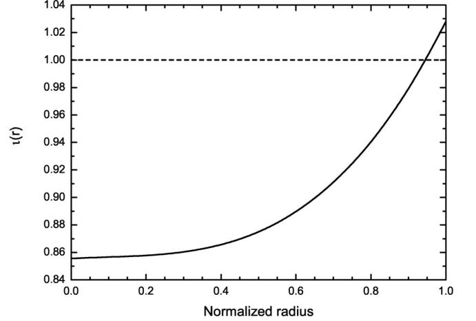
Fig. 4. Profile of rotational transform. The chain of 5 magnetic islands is created at the rational magnetic surface  $\iota = 1$  ( $r = 0.95$ ), when perturbation (3) is applied
