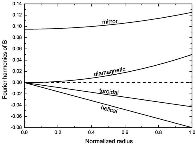
Fig. 2. Fourier harmonics of  $B$  for the high-mirror configuration
