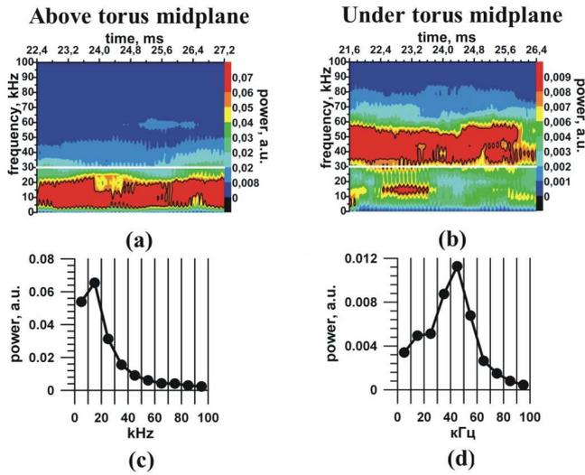
Fig. 3. Time evolution of fluctuation power spectra (a, b) and corresponding time-averaged spectra (c, d) in the top (a, c) and bottom (b, d) spacings of cross-section DD
