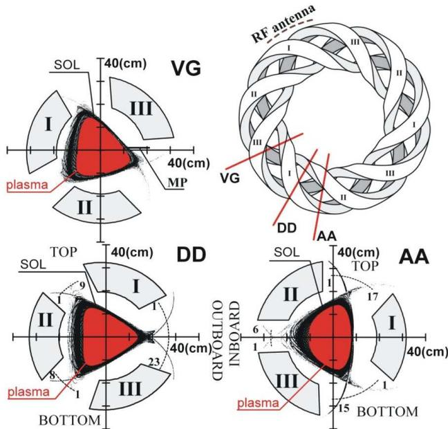
Fig. 2. Disposition of divertor probe arrays 1–17, 1–15, *etc.* (cross-sections AA and DD) and movable probe array (cross-section VG, segment MP) relative to helical coils I, II, and III and the calculated edge structure of field lines. Positions of 4 MP tips are shown in the inset to VG
