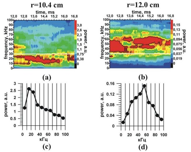
Fig. 4. Time evolution of fluctuation power spectra (a, b) and corresponding time-averaged spectra (c, d) in close vicinity to LCMS, a and c – MP position  $r = 10.4$  cm and more distantly; b and d –  $r = 12.0$  cm
