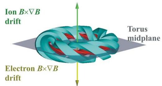
Fig. 1. Electron and ion  $\mathbf{B} \times \nabla B$  drift directions
