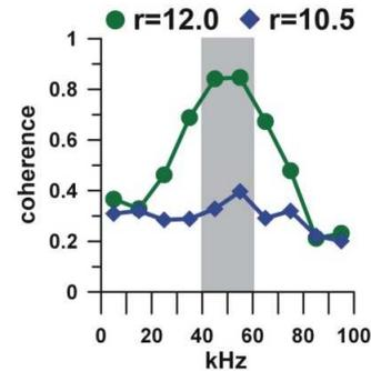
Fig. 5. Cross-coherence spectra for fluctuations in the divertor region (DD, bottom, probe N1, see Fig. 1) and the SOL (movable probe at  $r = 12.0$  cm and  $r = 10.6$  cm)
