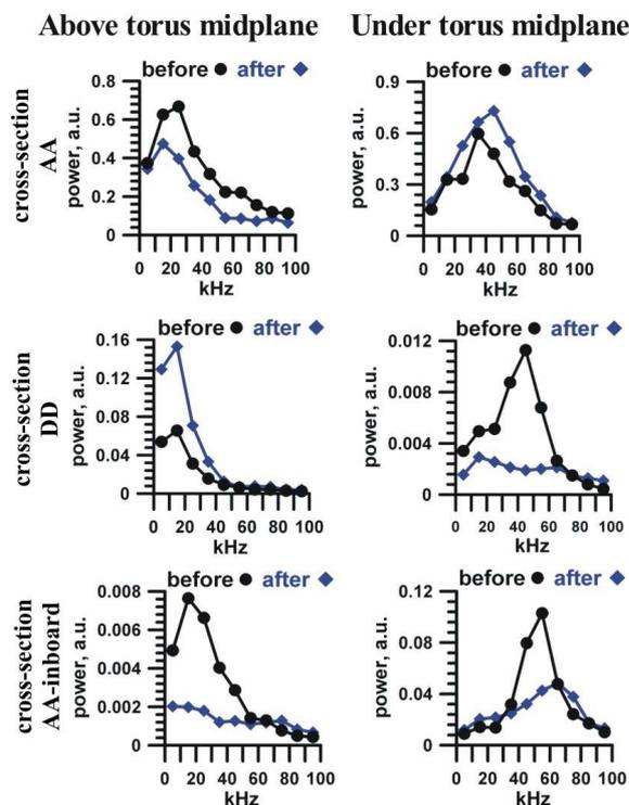
Fig. 6. Power spectra before and after the  $H$ -mode transition in two symmetric poloidal cross-sections AA and DD
