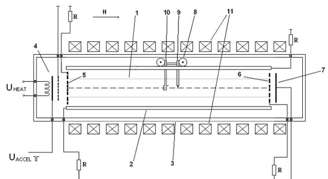
Fig. 1. Experimental installation: 1 – electron beam, 2 – drift chamber, 3 – vacuum chamber, 4 – injector, 5 – input grid, 6 – output grid, 7 – collector, 8 – mobile platform, 9 – Langmuir probe, 10 – electrostatic analyzer
