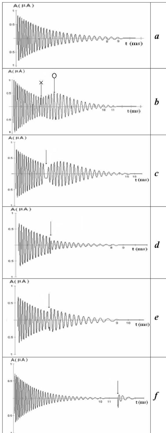
Fig. 2. Diocotron wave damping in the longitudinal magnetic field  $H = 1$  Oe. Arrow  $\times$  in panel *b* marks the point  $(t_{\min}, A_{\min})$ , arrow  $O$  in the same panel – the point  $(t_{\max}, A_{\max})$ , and arrows in panels *c* to *f* mark the moment of additional beam injection
