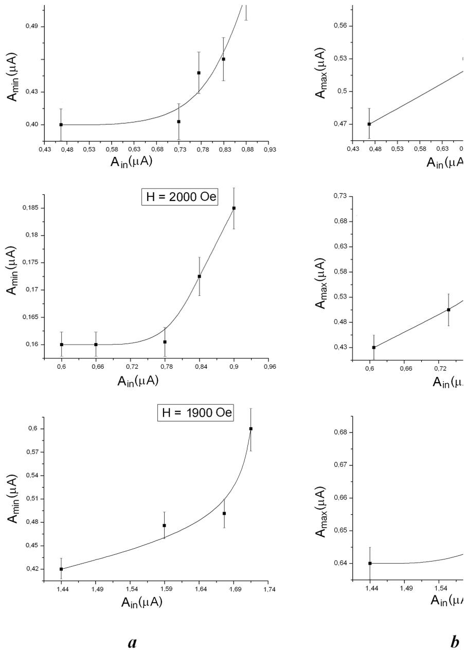
Fig. 3. Dependences of the minimal and maximal amplitudes on the initial one at the nonlinear damping of diocotron waves for various values of the longitudinal magnetic field strength
