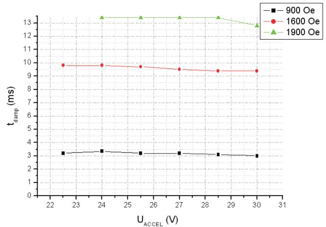
Fig. 5. Dependences of the time interval of the diocotron oscillation damping in the linear mode on the acceleration potential of the injector
