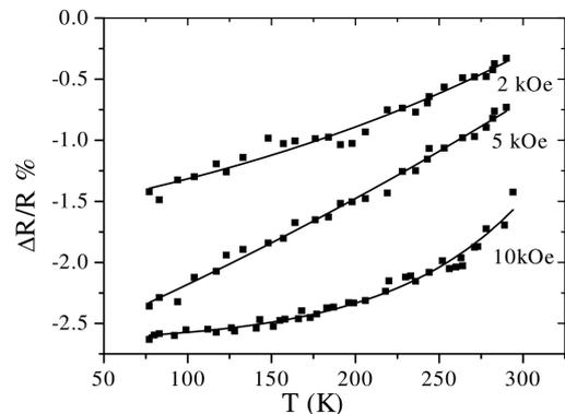
Fig. 4. Magnetoresistance of the Cu–Ni–Fe alloy as a function of the temperature in different magnetic fields
