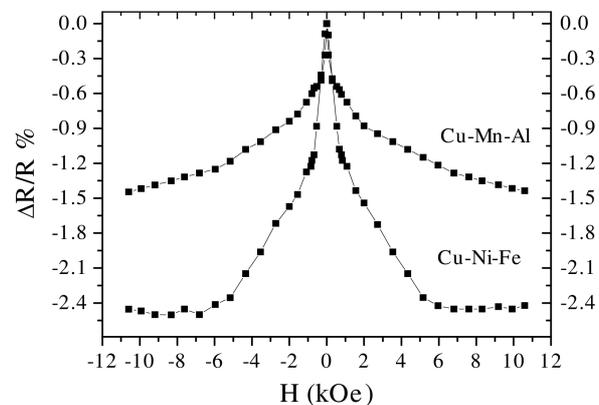
Fig. 5. Magnetoresistance of the Cu–Mn–Al and Cu–Ni–Fe alloys taken at  $T = 77$  K under a field parallel to the current
