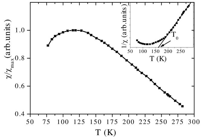
Fig. 1. Temperature dependence of the low-field ac magnetic susceptibility for the Cu–Mn–Al alloy. The inset shows the temperature dependence of the inverse susceptibility for the Cu–Mn–Al alloy
