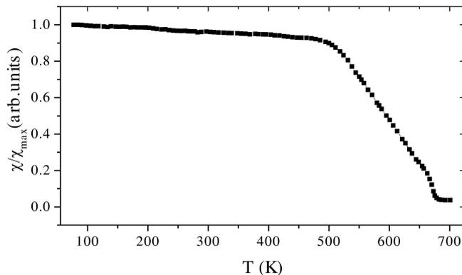
Fig. 2. Temperature dependence of the low-field ac magnetic susceptibility for the Cu–Ni–Fe alloy
