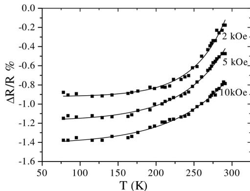
Fig. 3. Magnetoresistance of the Cu–Mn–Al alloy as a function of the temperature in different magnetic fields
