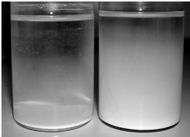
Fig. 10. Photos of \text{Al}_2\text{O}_3 water suspensions a) product of Al LTDF; b) product of Al+1% KCl LTDF
