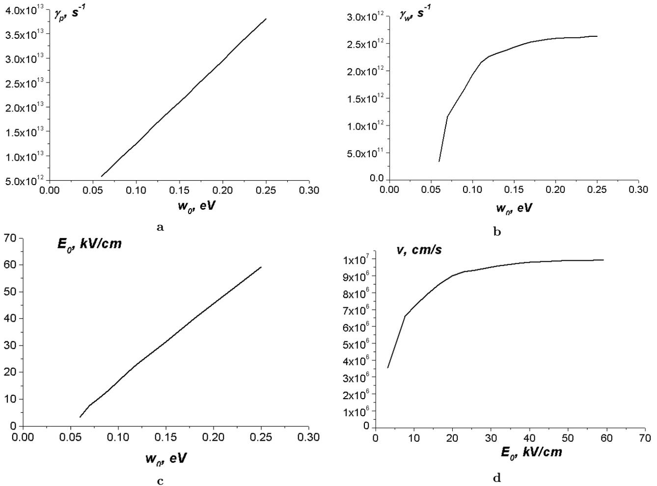
Fig. 1. Data used in simulations for silicon at room temperature of the lattice,  $T_{00} = 300$  K. Dependences of the momentum relaxation rate  $\gamma_p$  (a) and the energy relaxation rate  $\gamma_w(w)$  (b) on the average electron energy  $w$ ; the relation between the bias electric field  $E$  and  $w$  (c); the dependence of the drift electron velocity  $v$  on the bias electric field  $E$  (d)
