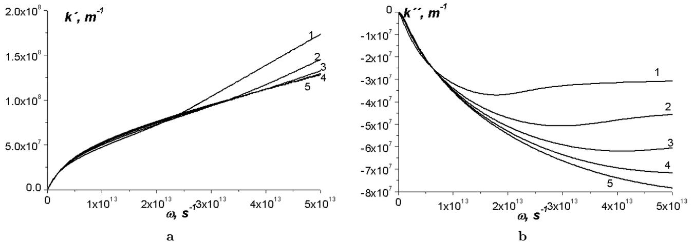
Fig. 4. Dependences of the real (a) and imaginary (b) parts of the wave number of space-charge waves on the frequency  $\omega$ ;  $n_0 = 10^{15} \text{ cm}^{-3}$ . Both the thermoconductivity and quantum corrections are taken into account. Curve 1 is at  $w_0 = 0.1 \text{ eV}$ , 2 is at  $w_0 = 0.15 \text{ eV}$ , 3 is at  $w_0 = 0.20 \text{ eV}$ , 4 is at  $w_0 = 0.25 \text{ eV}$ , and 5 is at  $w_0 = 0.30 \text{ eV}$
