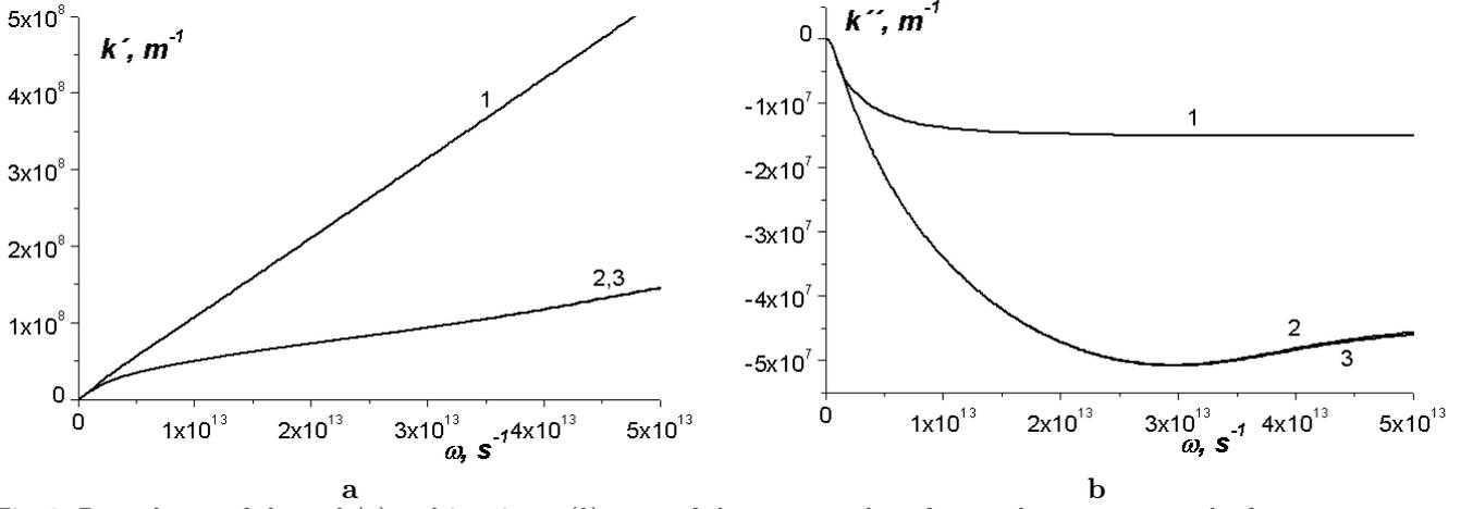
Fig. 2. Dependences of the real (a) and imaginary (b) parts of the wave number of space-charge waves on the frequency  $\omega$ ;  $n_0 = 10^{14} \text{ cm}^{-3}$ ,  $E_0 = 31 \text{ kV/cm}$  (the average electron energy is  $w_0 = 0.15 \text{ eV}$ ). Curve 1 is without both thermoconductivity and quantum corrections, curve 2 is with the thermoconductivity only, and curve 3 is with both the thermoconductivity and quantum corrections
