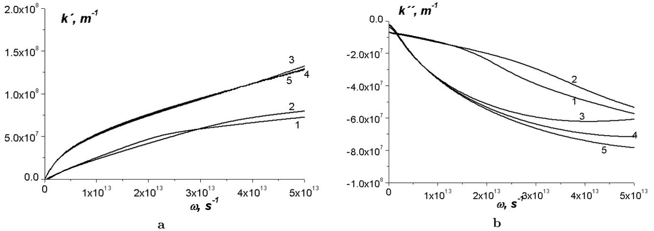
Fig. 5. Dependences of the real (a) and imaginary (b) parts of the wave number of space-charge waves on the frequency  $\omega$ ;  $n_0 = 10^{16} \text{ cm}^{-3}$ . Both the thermoconductivity and quantum corrections are taken into account. Curve 1 is at  $w_0 = 0.1 \text{ eV}$ , 2 is at  $w_0 = 0.15 \text{ eV}$ , 3 is at  $w_0 = 0.20 \text{ eV}$ , 4 is at  $w_0 = 0.25 \text{ eV}$ , and 5 is at  $w_0 = 0.30 \text{ eV}$
