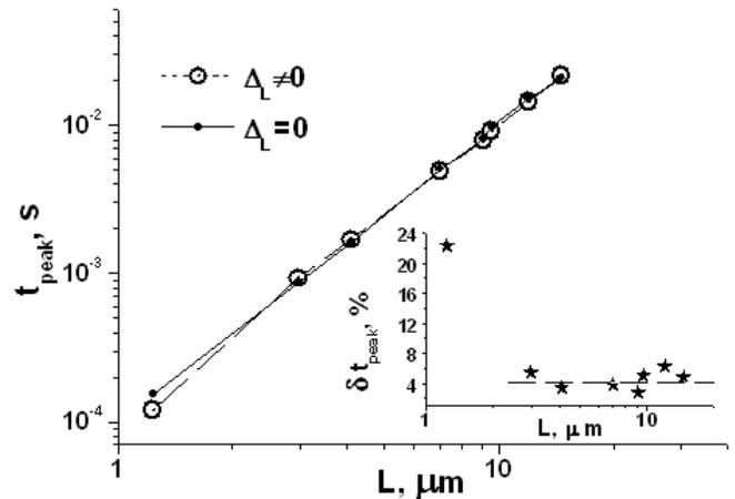
Fig. 4. Dependences of the position of  $t_{\text{peak}}$  on the thickness of a TiO<sub>2</sub> layer for the homogeneous ( $\Delta_L^i = 0$ ) and inhomogeneous ( $\Delta_L^i \neq 0$ ) distributions of the layer thickness. The insert shows the relative deviation of  $t_{\text{peak}}(\Delta_L^i = 0)$  from  $t_{\text{peak}}(\Delta_L^i \neq 0)$
