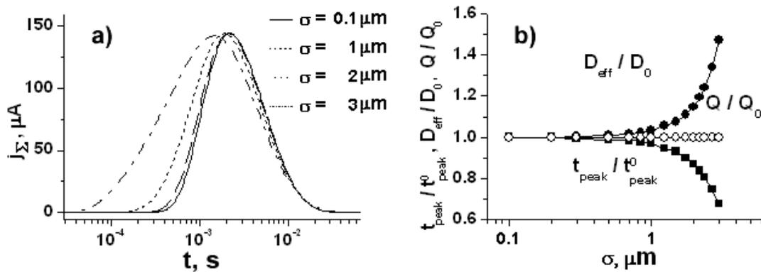
Fig. 3. *a* – Calculated photoresponse of the electrolyte/TiO<sub>2</sub>/FTO system for various values of the coefficient of dispersion of the thickness of a TiO<sub>2</sub> layer,  $\sigma$ ; *b* – dependence of  $D_{\text{eff}}$ , the position of the diffusion peak  $t_{\text{peak}}$ , and charge  $Q$  on the coefficient of dispersion of the thickness of a TiO<sub>2</sub> layer,  $\sigma$
