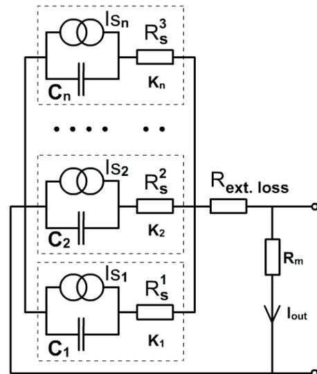
Fig. 2. Equivalent scheme of the electrolyte/TiO<sub>2</sub>/FTO system with regard for the inhomogeneity of a TiO<sub>2</sub> layer
