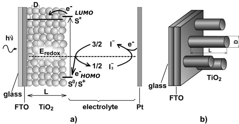
Fig. 1. *a*) Scheme of a solar cell with dye; *b*) model representation of a TiO<sub>2</sub> layer as the system of TiO<sub>2</sub> cylinders with a variable length and a constant diameter  $D$
