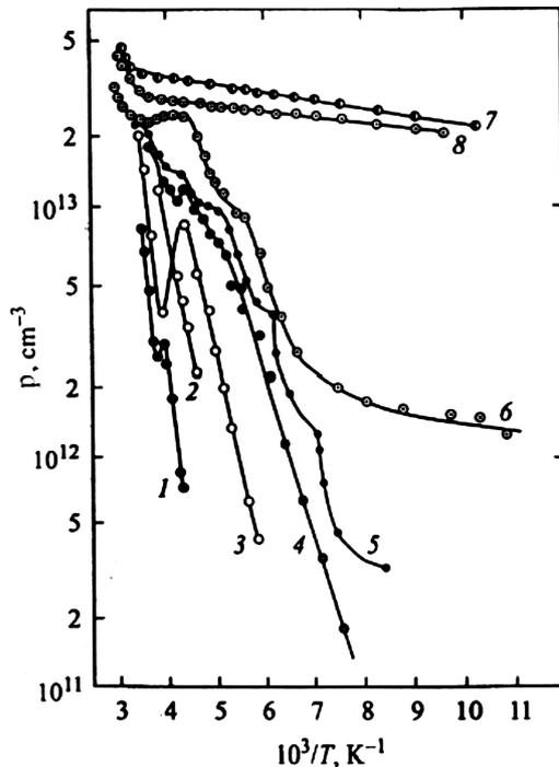
Fig. 1. Temperature dependences of the hole concentration  $p$  for a  $p$ -Si crystal irradiated with electrons for various annealing temperatures  $T_{\text{ann}}$ : before annealing (1), 100 (2), 170 (3), 240 (4), 270 (5), 300 (6), 400 (7), and 500 °C (8)
