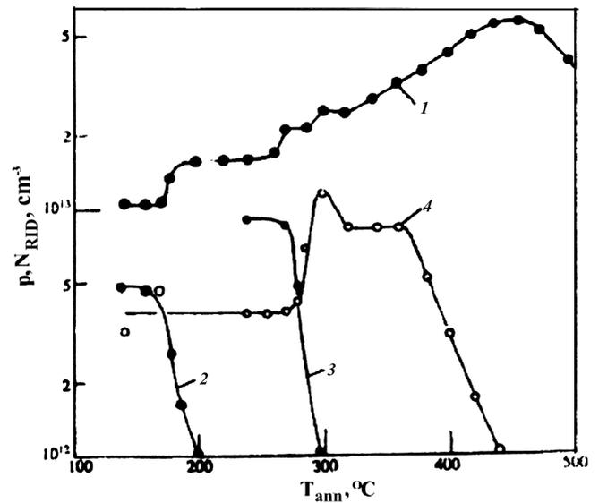
Fig. 2. Dependences of the hole concentration  $p$  (1) and some radiation-induced defects (2–4) on the isochronous annealing temperature in the  $p$ -Si crystals irradiated with electrons
