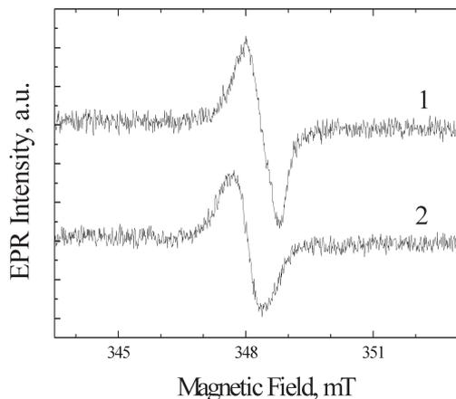
Fig. 1. EPR spectra of the  $\text{SiO}_x$  composite films annealed at 750 (1) and 1050 °C (2)
