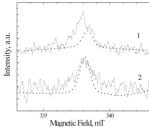
Fig. 2. ODMR spectra (solid lines) and integrated EPR spectra (dotted lines) of the  $\text{SiO}_x$  composite films annealed at 750 (1) and 1050 °C (2)
