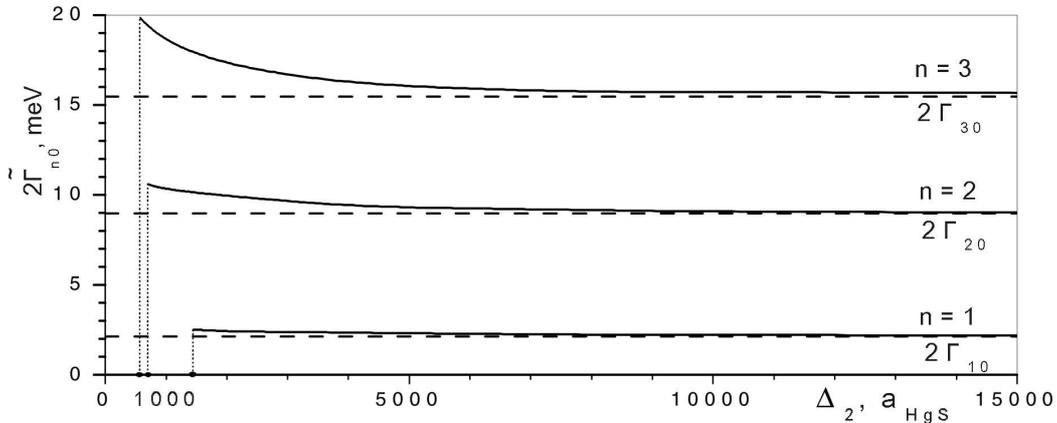
Fig. 5. Dependences of the discrete peak width  $2\tilde{\Gamma}$  of the quasistationary states on the thickness  $\Delta_2$  of the external well
