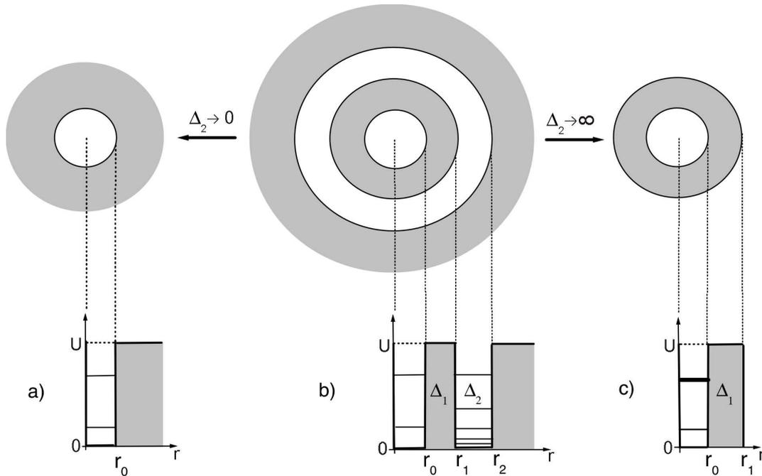
Fig. 1. Geometrical schemes of a simple closed (a), a closed double-well (b), and a simple open (c) spherical quantum dot (SQD), and the corresponding energy diagrams
