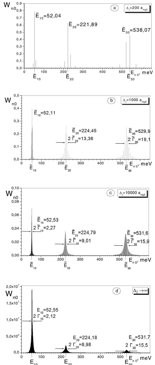
Fig. 4. Evolution of the probabilities  $\tilde{W}_{n0}$  for the electron to be located in two internal layers of a closed SQD and to possess the energy in the vicinity of the resonance ones (*a-c*), and the energy dependence of the probabilities  $W_{n0}$  in a simple open SQD (*d*)
