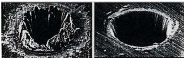
Fig. 1. 100-micron craters made in steel by a nanosecond pulse (left) and a femtosecond pulse (right) [1]
