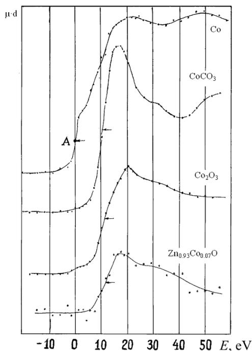
Fig. 1. Absorption spectra of Co ions in the thin  $\text{Zn}_{0.93}\text{Co}_{0.07}\text{O}$  film and in the reference specimens Co,  $\text{CoCO}_3$ , and  $\text{Co}_2\text{O}_3$
