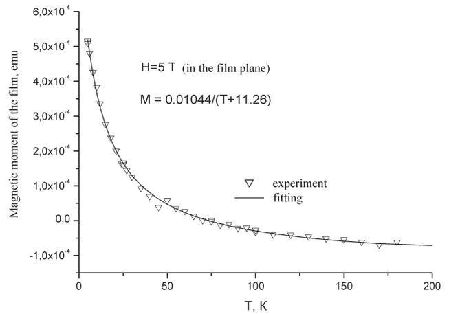
Fig. 3. Temperature dependence of the magnetic moment of the thin  $Zn_{0.93}Co_{0.07}O$  film in a 5-T magnetic field
