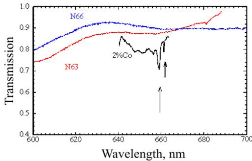
Fig. 2. Transmission spectra of the  $Zn_{1-x}Co_xO$  films with  $x = 0.036$  (N63) and  $0.078$  (N66), and a typical absorption spectrum of  $Co^{2+}$  in  $Zn_{1-x}Co_xO$  ( $x = 0.02$ )
