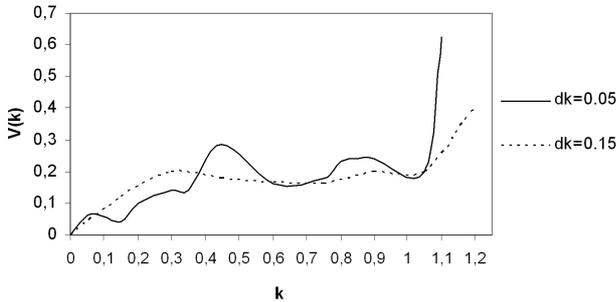
Fig. 3. Packet velocity versus the wave vector for different acceleration increments  $\Delta k$
