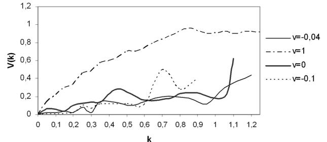
Fig. 4. Packet velocity versus the wave vector for different dispersion values  $v$
