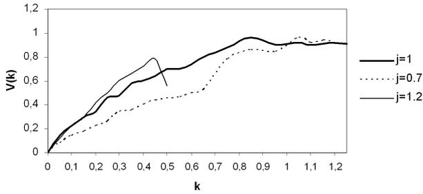
Fig. 5. Dependence of the packet velocity on the wave vector for different parameters  $j$  at  $v = 1$
