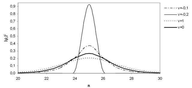
Fig. 2. Dependence of the square amplitude of the steady localized state on the phonon dispersion  $v$  at  $j = 1.2$
