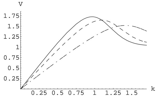
Fig. 9. Wave packet velocity versus  $k$  for different values of the parameter  $j$  at  $v = 1$
