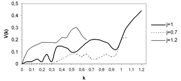
Fig. 7. Packet velocity versus the wave vector at  $v = -0,04$  for various values of the parameter  $j$
