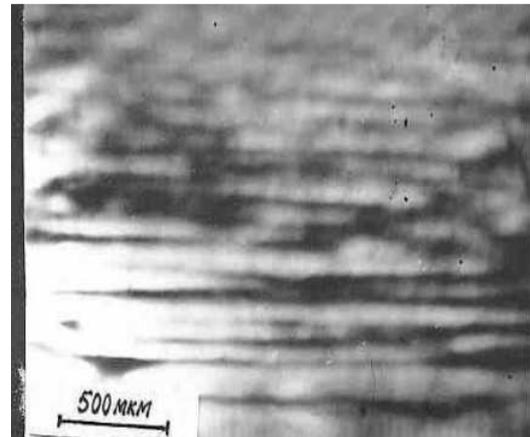
X-ray intensity distribution: *a* — original (as-received) molybdenum monocrystal, *b* — after diffusion of silicon into molybdenum, *c* — X-ray pattern before diffusion, *d* — after diffusion
