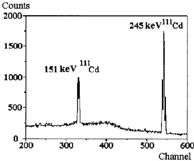
Fig. 1. Emission spectrum of an irradiated cadmium target
