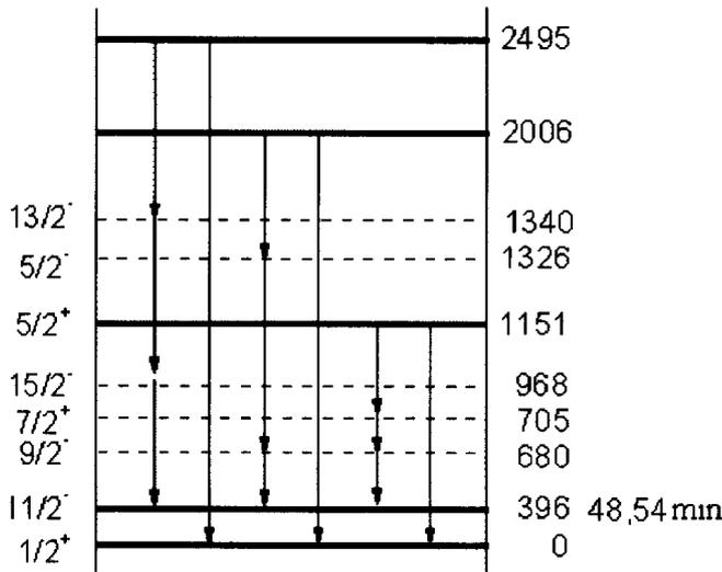
Fig. 3. Simplified schematic representation of the levels of a  $^{111}\text{Cd}$  nucleus
