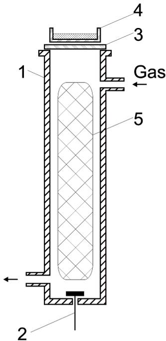
Fig. 1. Scheme of the experimental setup. 1 — chamber-cathode, 2 — anode, 3 — window made of KU-1 quartz, 4 — Petri dish made of KU-1 quartz, 5 — discharge plasma
