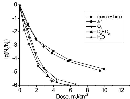
Fig. 6. Bacteria survival curves obtained at the treatment of an *Escherichia coli* suspension with  $2 \times 10^6$  CFU/ml density by UV radiation of a mercury lamp DB-30 and the radiation of discharges in air, oxygen, water vapor, and mixtures of deuterium with oxygen
