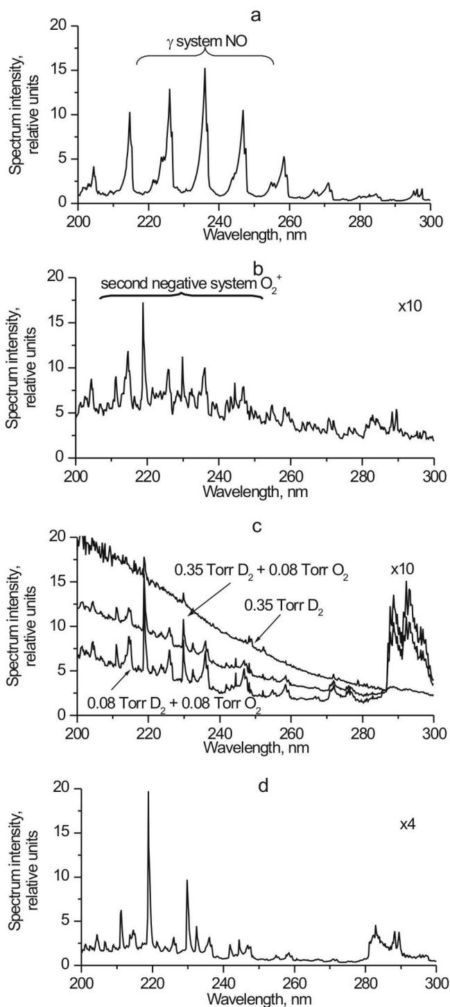
Fig. 3. UV radiation spectra of hollow-cathode discharge plasma on different working media: *a* — air, pressure 0.2 Torr, *b* — oxygen, pressure 0.1 Torr, *c* — mixture of deuterium and oxygen, *d* — water vapor, pressure 0.1 Torr
