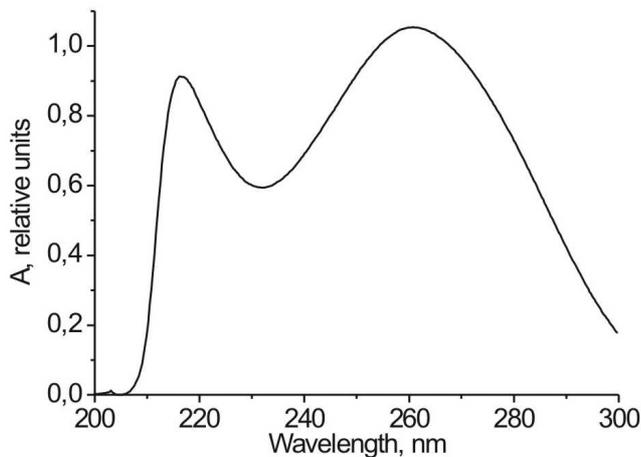
Fig. 2. "Weighing" curve obtained by multiplying the DNA absorption spectra and transmission curve of filter made of BaF<sub>2</sub> of 3 mm in thickness
