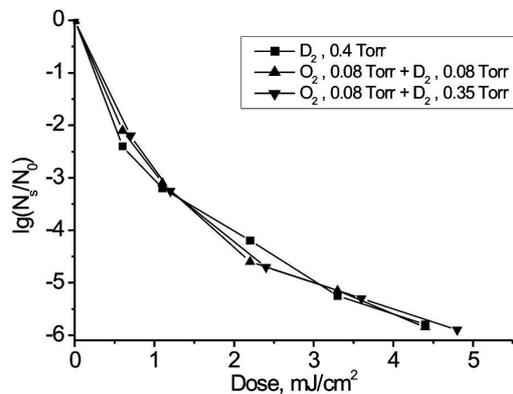
Fig. 5. Bacteria survival curves obtained at the treatment of an *Escherichia coli* suspension with  $10^6$  CFU/ml density by UV radiation of the discharge plasma on deuterium and mixtures of deuterium with oxygen
