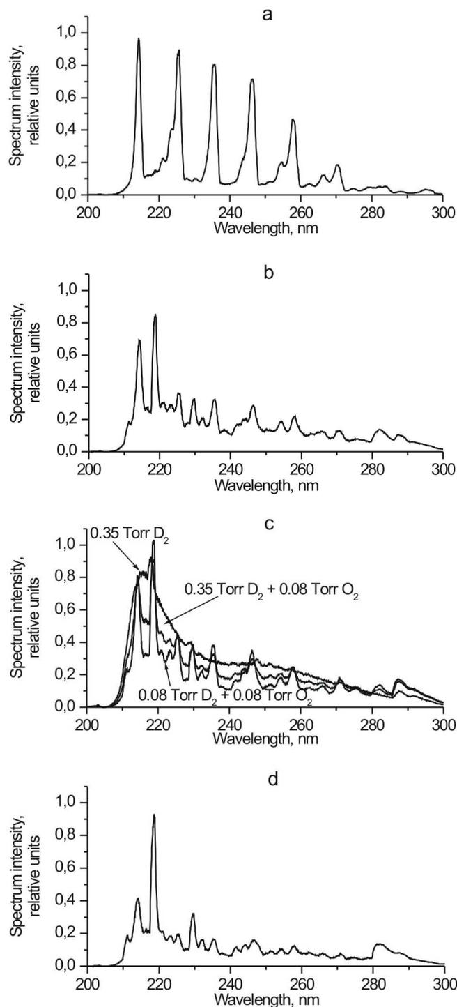
Fig. 4. Spectrum distribution of the “weighed” intensity of UV radiation of the discharge plasma on different working media: *a* — air, pressure 0.2 Torr, *b* — oxygen, pressure 0.1 Torr, *c* — mixture of deuterium and oxygen, *d* — water vapor, pressure 0.1 Torr
