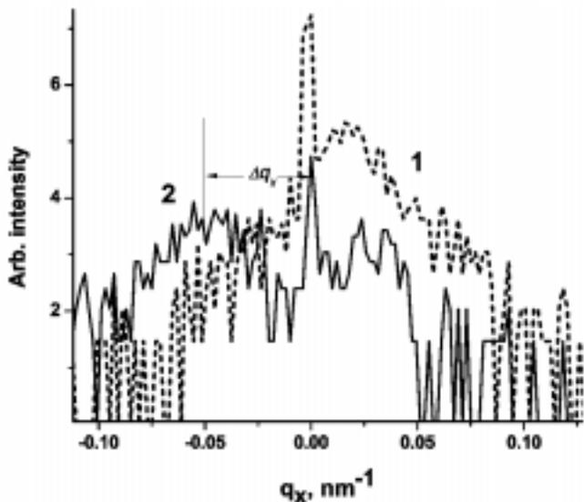
Fig. 4. Projections of the cross-sections of the diffuse scattering peaks around  $SL_0$  (1) and  $SL_1$  (2) satellites onto the  $q_x$  axis ( $\omega$  scans) calculated from the reciprocal space map for a 10-period SiGe/Si structure around point 224
