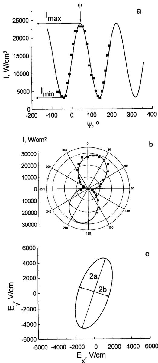
Fig. 4. Experimental (points) and theoretical (solid curves) dependences of the light intensity  $I_0$  at the back face of the crystal on the angle of polarizer rotation  $\psi$ , plotted in Cartesian (a) and polar (b) coordinates, and a view of the polarization ellipse (c). The theoretical curves were calculated by formulae (1) and (2). The polarization azimuth  $\varphi = 30^\circ$ .  $I_0 = 1.95 \times 10^5 \text{ W/cm}^2$
