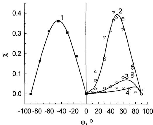
Fig. 6. Dependences of the ellipticity  $\chi$  of the polarization ellipse on the polarization azimuth  $\varphi$  for various values of the exciting light intensity  $I_0$  (the notations are the same as in Fig. 5). Curves 1–4 were calculated by formula (9), in which the values of  $I_{\min}$  and  $I_{\max}$  were determined by formula (1), where, in turn, the absorption factors  $K_{\perp}$  and  $K_{\parallel}$  were calculated by formula (2) and the angle  $\psi$  by formula (7)
