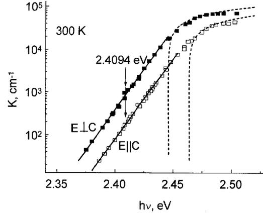
Fig. 2. Absorption spectra of a CdS single crystal. The number above the arrow indicates the photon energy of a laser emission, for which the influence of the light intensity on the light polarization state was investigated. Dashed curves correspond to the approximations of the dependences  $K_{\perp}(h\nu)$  and  $K_{\parallel}(h\nu)$  by the root law. Solid lines denote the Urbach sections of the corresponding absorption spectra
