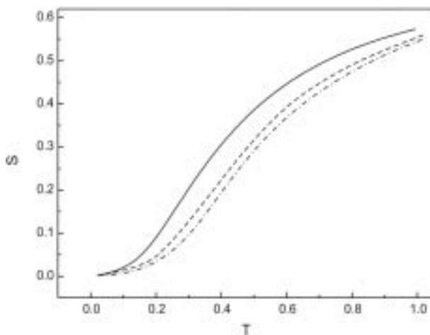
Fig. 3. Dependences  $s(T)$  at  $\rho = 1/2$ ,  $v(r) = 1/r$ , and various  $M$ . The continuous curve corresponds to  $M = 1$ , the dashed one — to  $M = 2$ , and the dash-dotted line — to  $M = 3$
