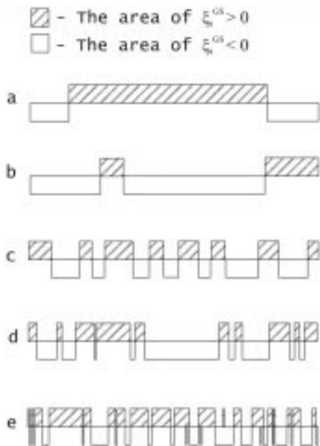
Fig. 5. Examples of the GS configurations of a 1D WGDHL corresponding to the chain including  $10^4$  sites (a–d) and 400 sites (e) and various values of  $\rho$ : a –  $\rho = 0.25$ , b – 0.3, c – 0.4, d – 0.45, e – 1
